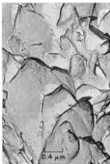
Fig. 8 Palladium-shadowed plastic-carbon replica of a fracture in nickel showing reticulated shadowing metal on dimples. Reticulation was caused by the melting of the shadowing metal in the microscope and the formation of globules. 22,500×
