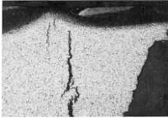
Fig. 174 Polished and etched section taken from location A in Fig. 172, showing the arc strike visible at the left arrow in Fig. 173. The large cracks present here are extensions of the fracture, which is visible in profile at right. Nital etch, 7×
