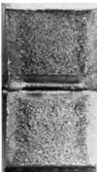
Fig. 1215 Specimen aged at 800 °C (1470 °F) 2 h and air cooled. Unlike Fig. 1213, this fracture shows little deformation, and impact energy was less than 27 J (20 ft · lb). See also Fig. 1216. 4.8× (Figures 1207, 1208, 1209, 1210, 1211, 1212, 1213, 1214, 1215, 1216, 1217, and 1218 present six related pairs of light and SEM fractograph of specimens of an Fe-12Ni-0.5Ti alloy intended for use at cryogenic temperatures. The series shows the effect on Charpy impact energy at -196 °C (-321 °F), and on fracture-surface characteristics, of the temperature of aging after austenitizing at 900 °C (1650 °F) for 2 h and air cooling.)
