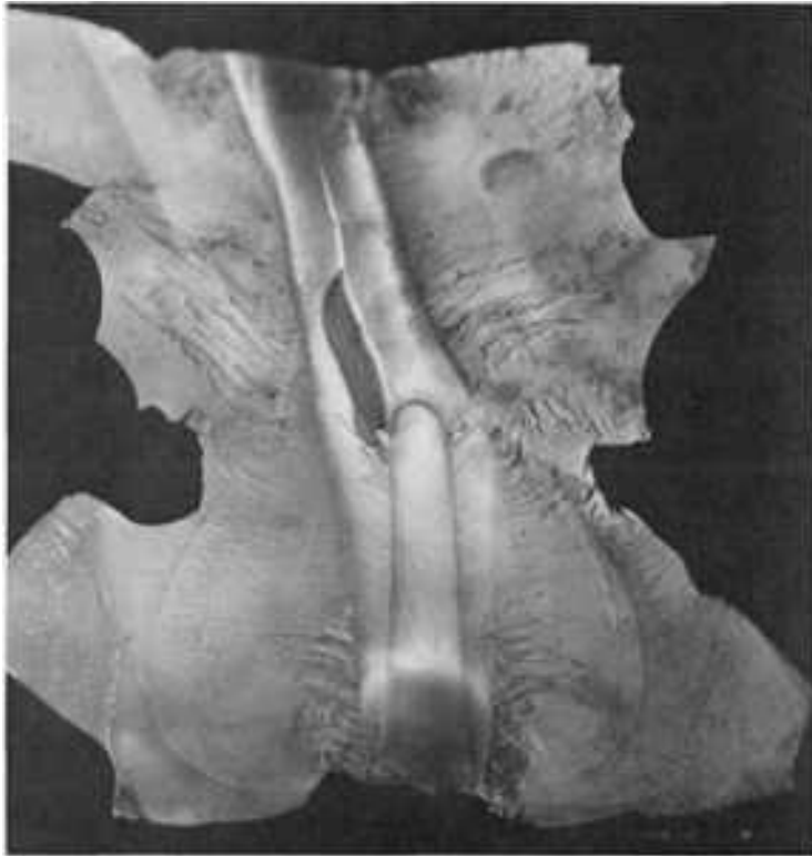
Fig. 65 Macrograph showing a line spall that broke off a forged, hardened alloy steel roll. The central region of the fracture shows evidence of crack growth by fatigue. Final rupture occurred by brittle fracture. See also Fig. 66. 0.65×
