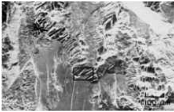
Fig. 1058 Corrosion-fatigue fracture in aluminum alloy 7475-T6 tested in a 3.5% NaCl solution under a cyclic stress-intensity range ( \Delta K ) of 13 \text{ MPa}\sqrt{m} ( 12 \text{ ksi}\sqrt{in} ) at 10 cps, showing contrasting features: ductile striations (unresolved) in smooth regions; brittle striations in adjacent grains. See also Fig. 1059. SEM, 100×
