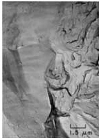
Fig. 401 TEM p-c replica taken at the root of the quench crack, marked A, in Fig. 397, and the beginning of the impact fracture, marked B there. At left are the last vestiges of intergranular cracking, and at right is the beginning of quasi-cleavage cracking in this very brittle specimen. 6500×
