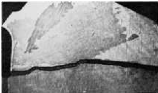
Fig. 841 A macroetched view of a cracked turbine-rotor blade near the arrow in Fig. 839, displaying large columnar grains and a crack that initiated at the trailing edge (at left in this view) of the blade. This crack appears to have followed an intergranular path. Etched in 95 parts conc HCl, 5 parts 35% \text{H}_2\text{O}_2 . 5.5×
