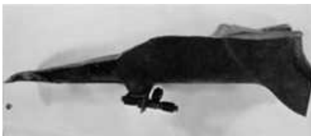
Fig. 1074 Side view of a piece of fractured aluminum alloy 7079-T6 bogie beam of an aircraft main landing gear. The fracture surface is at top, in profile. The very straight edge at lower right is a saw cut that was made to separate the fracture area from the remainder of the beam to facilitate inspection. Hardness of the beam was 84 HRB. See also Fig. 1075 and Fig. 1076. 0.25×
