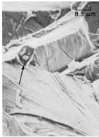
Fig. 1202 Higher-magnification view of the slow-bending fracture in Fig. 1201. During testing, specimen temperature was controlled by an isopentane bath cooled with liquid nitrogen. Ferrite grain size, 30 \mu\text{m} . The angle of the notch was 45°, and the nominal radius of the root of the notch was 0.25 mm (0.01 in.). The fracture originated at cracked Ti(C, N) particles (as at arrow). SEM, 1200 \times
