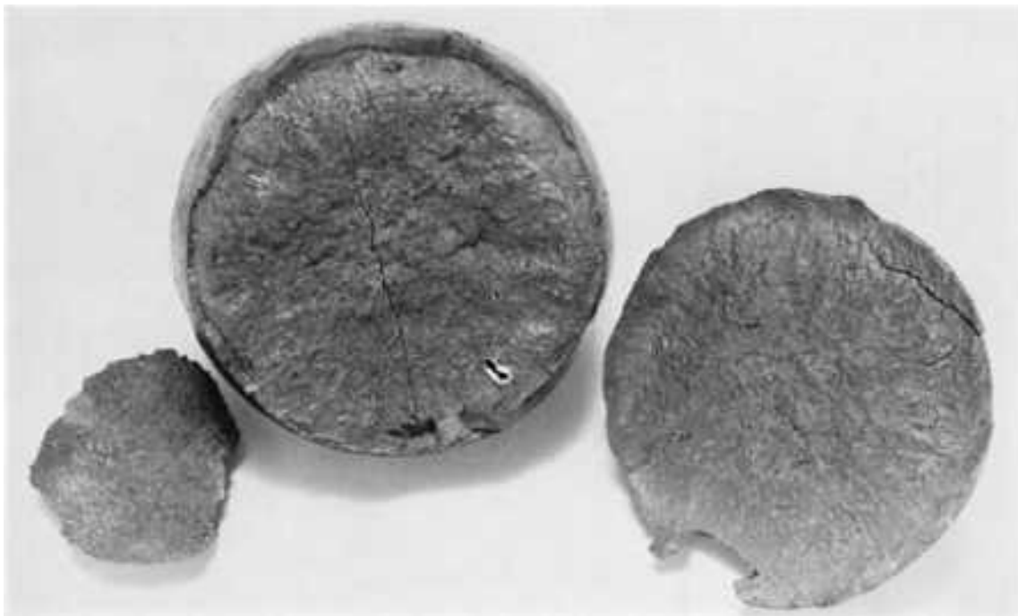
Fig. 542 Catastrophic failure of 75-mm (3-in.) diam manganese steel grinding ball after 51,440 severe ball-on-ball impacts in a laboratory test. Composition: 1.21% C, 5.3% Mn, 1.8% Cr, 1.1% Mo, 0.46% Si, 0.1% Ni, and 0.1% Cu. Fracture initiated at an interior crack. (Note another such crack on the fracture surface at center.) The interior of the ball was under tension. The outer rim was under compression due to heat treatment and plastic deformation from impacts. (H.W. Leavenworth, Jr., U.S. Bureau of Mines).
