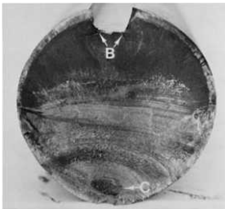
Fig. 51 Macrograph of the fracture face of an AISI 4320 drive shaft that failed by fatigue. The failure began at the end of a keyway that was machined without fillets (B) and progressed to final rupture at (C). The final rupture zone is small, indicating that loads were low.
