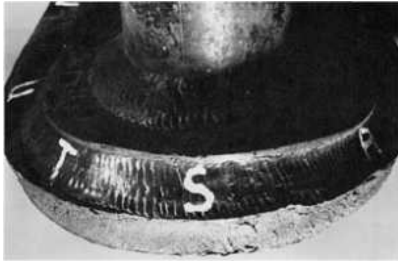
Fig. 179 View of the flange in Fig. 177, showing an adjacent area of the fracture surface of the pressure-vessel shell. Although not as discernible here as in Fig. 184, chevron marks throughout the fracture surface clearly point toward the area at S, and subsequent examination identified the toe of the flange weld at S as the crack nucleus. ~0.3×
