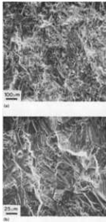
Fig. 8 Secondary electron images of the fatigue-precracked region of an alloy X-750 test specimen. (a) 65 \times . (b) 260 \times
