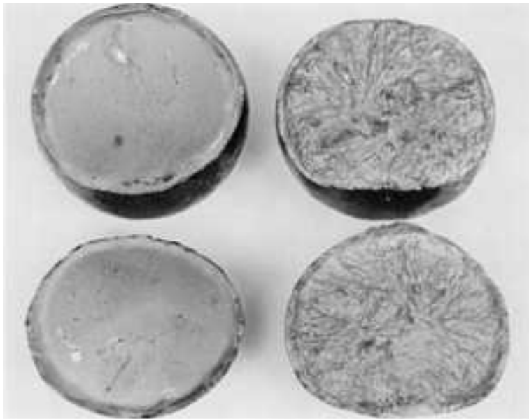
Fig. 541 Mating fracture surfaces of commercial 75-mm (3-in.) diam grinding balls. Fracture was caused by severe ball-on-ball impacts in laboratory tests. Left top and bottom: Commercial forged and heat-treated low-alloy steel ball. Composition: 0.63% C, 0.90% Mn, 0.76% Si, 0.66% Cr, 0.018% P, and 0.011% S. Right top and bottom: Experimental manganese steel ball, cast and heat treated. Composition: 0.97% C, 5.3% Mn, 1.9% Cr, 1.0% Mo, 0.48% Si, 0.03% P, and 0.018% S. Outer rim of ball was under compression due to heat treatment and plastic deformation from impacts. (H.W. Leavenworth, Jr., U.S. Bureau of Mines)
