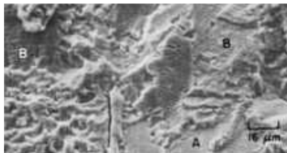
Fig. 1048 Corrosion-fatigue fracture in aluminum alloy 7075-T6 tested in a 3.5% NaCl solution. During testing, specimen was subjected to an applied electrical potential of -0.700 mV as measured against a standard calomel electrode. A mixture of ductile striations (at A) and brittle striations (at B) is evident, with some fissures. See also Fig. 1049. SEM, 625×
