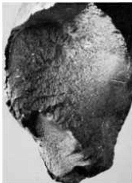
Fig. 263 Higher-magnification view of fracture surface in Fig. 262. The fatigue crack began at subsurface origin (at arrow), not at a surface defect. Final fast fracture formed shear lips at top, at left, and at bottom. 15×
