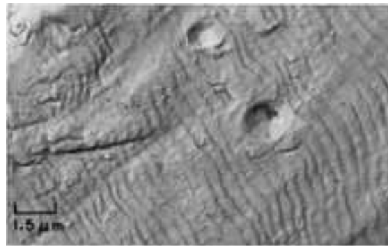
Fig. 624 TEM p-c replica of an area at C, about 4.4 mm (0.175 in.) from the notch, in Fig. 618. Note that the fatigue striations here are more widely spaced than those in Fig. 623, which indicates that the effective stress increased as the crack penetrated into the specimen. Partly formed dimples are visible above and right of center. 6500×
