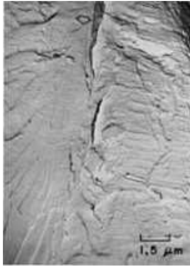
Fig. 1198 TEM p-c replica of another area at A in Fig. 1196. Fine, roughly horizontal striations are visible in a fatigue patch at the arrow at top center; the marks at the right include widely spaced horizontal fissures. 6500×
