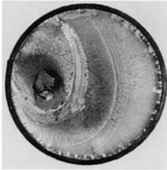
Fig. 218 Fatigue-fracture surface of an AISI 1050 shaft (35 HRC) subjected to rotating bending. Numerous ratchet marks (small shiny areas at surface) indicate that fatigue cracks were initiated at many locations along a sharp snap-ring groove. The eccentric pattern of oval beachmarks indicates that the load on the shaft was not balanced. The final rupture area is near the left (low stress) side, where there may have been no fatigue action. (D.J. Wulpi, Consultant)
