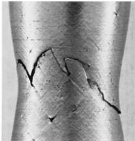
Fig. 123 Tensile-test fracture in a 13-mm (0.505-in.) diam specimen of cast 0.20% C steel with hardness of 255 HB. Note that pronounced 45° shear deformation has produced shear lips and also numerous secondary cracks, which formed at pores. 7.5×
