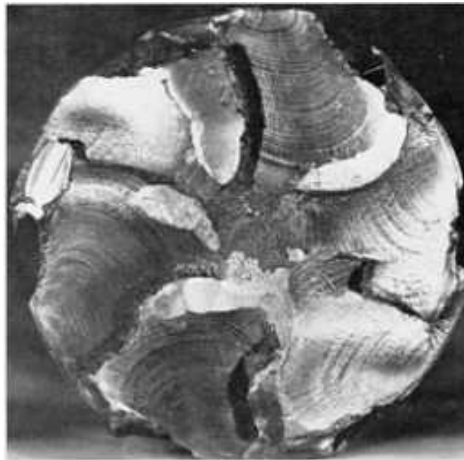
Fig. 476 Surface of a fatigue fracture that began at six fillet areas around the periphery of a shaft, near the runouts of spiral grooves. The material is AISI 4817 steel; the shaft was carburized and heat treated to a surface hardness of 60 HRC. The fatigue cracks penetrated equally, indicating that stress concentrations at the six fillet areas were essentially equal. \sim 2.13\times
