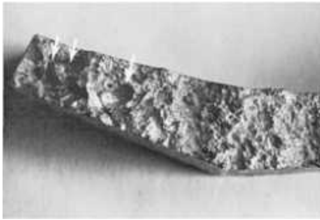
Fig. 923 This fracture surface is from the bracketed edge of the sand-cast carrier tray in Fig. 921. Like the surface shown in Fig. 922, the one here exhibits the characteristics of brittle fracture, there being no sign of a shear lip at any of these edges. Again, there is evidence of porosity; the arrows point to quite large gas cavities. The cavities could have been caused by a reaction between the liquid metal and organic binders in the sand mold, or could have resulted from entrapped air being carried into the mold by undue turbulence in pouring the casting. 3×
