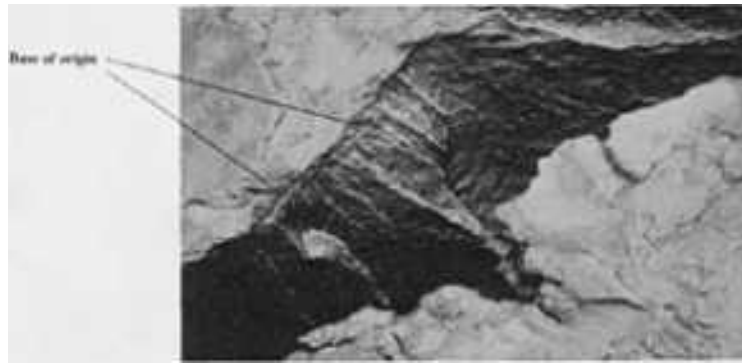
Fig. 498 Fatigue crack origin on surface of spring was intentionally opened to reveal details of fracture initiation. Material: modified AISI 5160 (0.5% Cr, 0.1 to 0.2% V) wire. The spring was tested in the laboratory at stresses well in excess of those normally encountered in service. The surface-breaking portion of the fatigue origin is indicated on the fractograph. It initially appeared under the SEM as a faint line, transverse to the wire at the center, with each end at a slight angle. After intentional opening (see fractograph), the origin was shown to be roughly triangular in shape and defined by vertical ridges extending into the material. The balance of the fracture surface has a typical tensile failure pattern. SEM, 590 \times (J.H. Maker, Associated Spring, Barnes Group Inc.)
