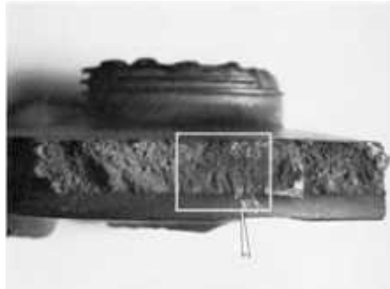
Fig. 835 Segment of a fractured second-stage gas-turbine wheel, cast from alloy 713C, that broke from fatigue in service. (About half of the disk portion of the wheel was never recovered.) The fracture origin (at arrow) was in a grinding-relief groove adjacent to the wheel-balancing pad. Additional circumferential cracks, not adjuncts of fracture, were found elsewhere in the grinding-relief groove. See Fig. 836 for a higher-magnification view of the rectangular area. 2 \times
