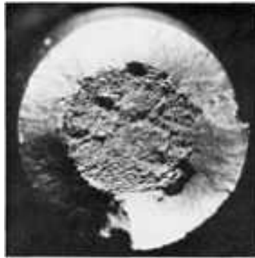
Fig. 24 Tensile fracture of a 4340 steel specimen tested at 120 °C (250 °F). The fracture contains a fibrous zone and a shear-lip zone. The steel microstructure consisted of tempered martensite; hardness was 46 HRC. The fracture started at the center of the fibrous zone, which shows circumferential ridges. The outer ring is the shear-lip zone. About 11×
