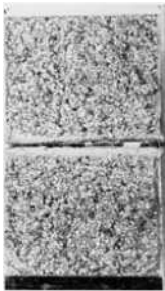
Fig. 1209 Both fracture surfaces of a specimen aged at 650 °C (1200 °F) 2 h and air cooled. See also Fig. 1210. 4.8× (Figures 1207, 1208, 1209, 1210, 1211, 1212, 1213, 1214, 1215, 1216, 1217, and 1218 present six related pairs of light and SEM fractograph of specimens of an Fe-12Ni-0.5Ti alloy intended for use at cryogenic temperatures. The series shows the effect on Charpy impact energy at -196 °C (-321 °F), and on fracture-surface characteristics, of the temperature of aging after austenitizing at 900 °C (1650 °F) for 2 h and air cooling.)
