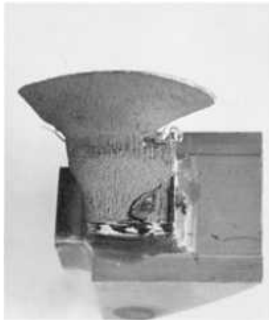
Fig. 337 Mating fracture surface to that shown in Fig. 336. There appears to be no evidence of fatigue marks; however, fatigue cracking may have taken place within a very small area at the crack origins. Fracture was evidently caused by a sudden overload. See also Fig. 338. Actual size
