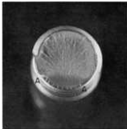
Fig. 781 Low-cycle fatigue fracture in threaded specimen of AISI H11 tool steel (same heat treatment and tensile strength as in Fig. 774) that broke after 21,000 cycles of tension-tension ( R = 0.1 ); maximum load, 60% of tensile strength. Region A-A is fatigue portion of fracture. See also Fig. 782, 783, 784, and 785. 6 \times
