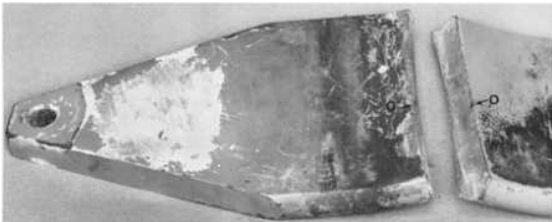
Fig. 499 Fatigue fracture in an AISI 6150 steel spring leg of an aircraft main landing gear, heat treated to a minimum tensile strength of 1550 MPa (225 ksi) and a hardness of 49 HRC. Visual inspection of the fracture surfaces showed that the fatigue crack originated at the location marked by arrows O. The appearance of the external surface of the spring leg indicated that the part had been shot peened, but that peening had been inadequate. The dimensions of the spring leg conformed to specifications. See also Fig. 500, 501, 502, 503, and 504. 0.6 \times
