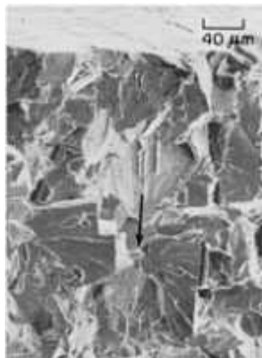
Fig. 1201 Surface of a slow-bending fracture produced at -160 °C (-256 °F) in Fe-3.9Ni alloy deoxidized with aluminum and titanium, which was forged at 1260 °C (2300 °F), hot rolled at 1040 °C (1905 °F), annealed at about 1000 °C (1830 °F), and air cooled. Root of specimen notch is at top. Fracture was by cleavage that began at cracked Ti(C,N) particles (as at arrow). See also Fig. 1202. SEM, 250×
