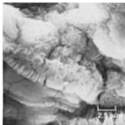
Fig. 738 Another higher-magnification view of the crack-origin area of the SCC fracture surface shown in Fig. 735, displaying a coating of a hydroxide corrosion product containing many fine secondary cracks. Compare with the area shown in Fig. 737. SEM, 4000×
