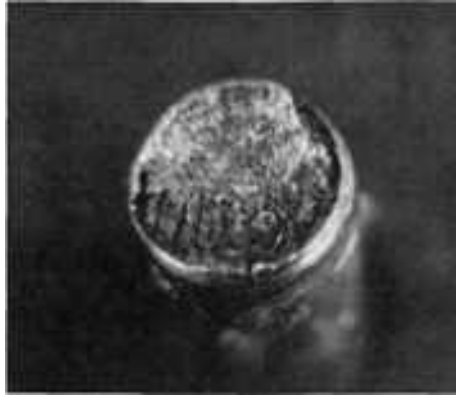
Fig. 794 Fracture caused by stress-corrosion cracking in a threaded specimen of AISI H11 tool steel (same heat treatment and tensile strength as in Fig. 786) at a sustained loading of 75% tensile strength in a 3.5% NaCl environment at room temperature. Appreciable corrosion is evident. See also Fig. 795, 796, and 797. 6×
