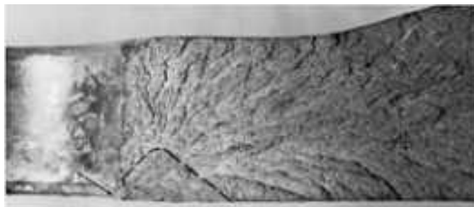
Fig. 1080 Fracture surface inboard of the bolthole in the clevis-attachment lug in Fig. 1079. The primary stress-corrosion crack, which originated at arrow, is within the area enclosed by the dashed line (lower left). The remainder of this surface shows chevron marks typical of final fast fracture. 4×
