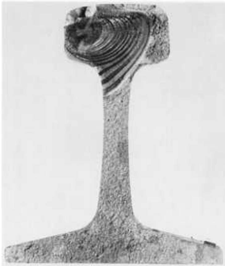
Fig. 70 Macrograph of a rail that contained a detail fracture (upper left, beneath the rail head surface) that was placed in service in the FAST test track. Note the fatigue fracture that grew from the detail fracture. 0.75×. (R. Rungta, Battelle Columbus Laboratories)
