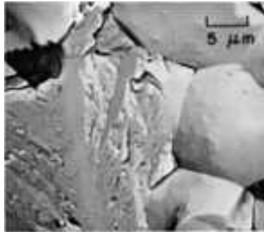
Fig. 1235 Impact fracture in sintered tungsten that had been recrystallized, showing separated-grain facets (at right) and cleavage facets (at left); the cleavage facets exhibit twins in the {112} plane. TEM p-c replica, 2000×
