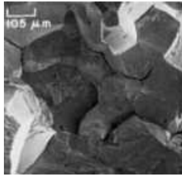
Fig. 874 Fracture in Duranickel that, except for being aged 4 h, was heat treated and tested same as Fig. 872. Fracture here is more completely intergranular, with less cleavage, than Fig. 872. Both fractures show secondary cracks. See also Fig. 875. SEM, 95×
