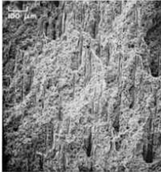
Fig. 338 Magnified view of the fracture surface in Fig. 336, taken at an area away from the edge, and showing the dimples that are typical of transgranular fast fracture. Vertical marks are sulfide stringers. SEM, 100×
