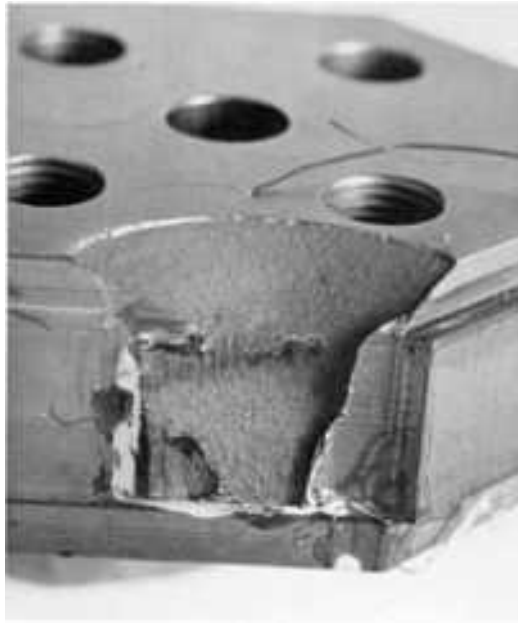
Fig. 336 Fracture surface of a broken AISI 4140 steel load cell. The radial marks indicate that two crack origins formed at the bottom surface of the cell, apparently near the toe of a weld. Note the continuous shear lip around the top edge. See also Fig. 337 and 338. Actual size
