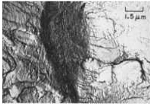
Fig. 622 TEM p-c replica of a sixth area near A in the fracture surface in Fig. 618, showing distinct fatigue striations. The markings to the right of the dark region are believed to be cleavage steps, not fatigue striations. 6500×
