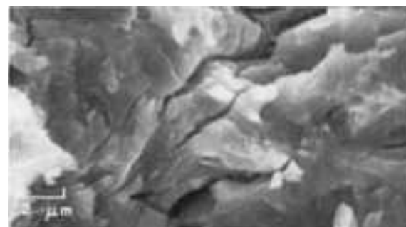
Fig. 1151 View of the fracture surface in Fig. 1150, seen at higher magnification, which shows in greater detail the fine secondary cracks; these are transgranular, in contrast to the network of major secondary cracks. (Structure is continuous \beta phase with dispersed \alpha phase.) The fracture is brittle, but the facets are small and
