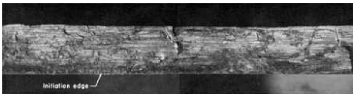
Fig. 1060 Surface of a fracture in an aircraft lower-bulkhead cap fabricated from an extrusion of aluminum alloy 7075-T6. The cap was cut open to expose the fracture for inspection, and evidence of corrosion was found along the edge at which fracture was initiated (bottom edge in this view). Secondary cracks had produced "leaves" (at arrows) in the fracture surface. See also Fig. 1061, 1062, 1063, 1064, 1065, 1066, 1067, 1068, and 1069. 8×
