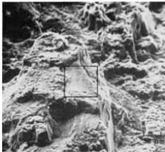
Fig. 986 Fracture surface of a fatigue-test specimen of aluminum alloy 2024-T3 that was tested in an environment of a 3.5% solution of NaCl in water. The stress-intensity range ( \Delta K ) was 19.8 \text{ MPa}\sqrt{m} ( 18 \text{ ksi}\sqrt{in} ) at 10 cps. The central region of this view contains patches of well-defined fatigue striations. In adjacent regions, there appear to be faintly defined striae that have been obscured by corrosion. In other regions, it is uncertain whether fatigue or cleavage was active. See Fig. 987 for area in rectangle. SEM, 260×
