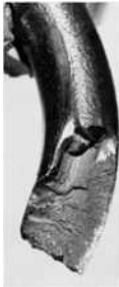
Fig. 271 Surface of a complex fatigue fracture in a valve spring formed from AISI 1070 steel wire, showing two facets at right angles. 8×
