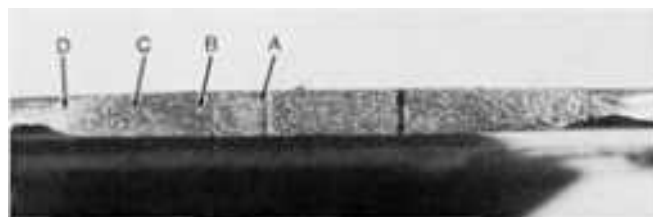
Fig. 618 Surface of a high-cycle fatigue fracture in a notched specimen of AISI type 302 stainless steel sheet subjected at 425 °C (800 °F) to tensile stress cycled from 24.8 to 124 MPa (3.6 to 18 ksi) at 1000 cycles/min. Fracture occurred after 1,625,450 cycles. The notch in the specimen was a center hole 0.25 mm (0.01 in.) in radius and 5 mm (0.20 in.) wide. Fatigue area became purple; fast-fracture area became straw colored, with shear and necking. See Fig. 616, 617, 619, 620, 621, 622, 623, 624, 625, and 626 for views at A, B, C, and D. 5×
