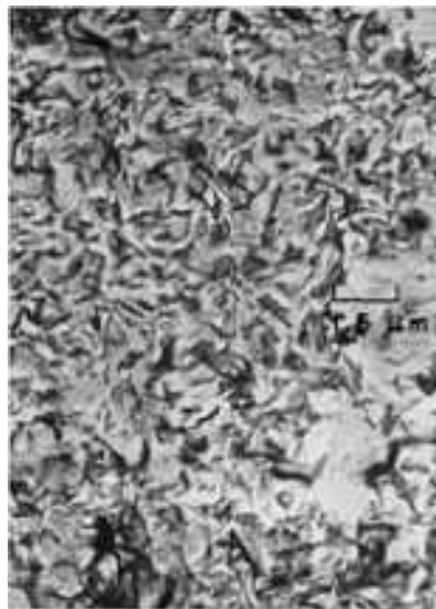
Fig. 1199 TEM p-c replica of an area at B in Fig. 1196. In this area, the fracture surface is largely obscured by corrosion products. The few facets that are visible have essentially no distinguishable features. 6500×
