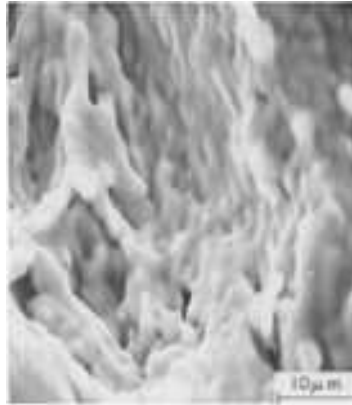
Fig. 73 Effect of temperature on the fracture of an ultralow-carbon steel. The 0.05C-0.82Mn-0.28Si steel containing 180 ppm S was annealed for 5 min at 1425 °C (2620 °F), cooled to 950 °C (1740 °F), and held for 3 min before tensile testing at a strain rate of 2.3 \times 10^{-4} \text{ s}^{-1} . The fracture, which occurs by dimple rupture when tested at room temperature, exhibits intergranular decohesion at 950 °C (1740 °F). Source: Ref 209
