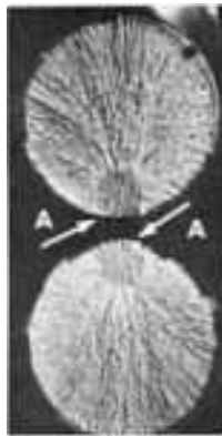
Fig. 757 Mating fracture surfaces of eccentrically loaded tensile specimen of A4N tool steel. Note fibrous zones of initial fracture (A). 2.25×
