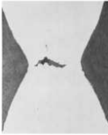
Fig. 23 Initiation of fracture in a tensile-test specimen. Note that the fracture initiated at the center of the specimen 4.75 ×
