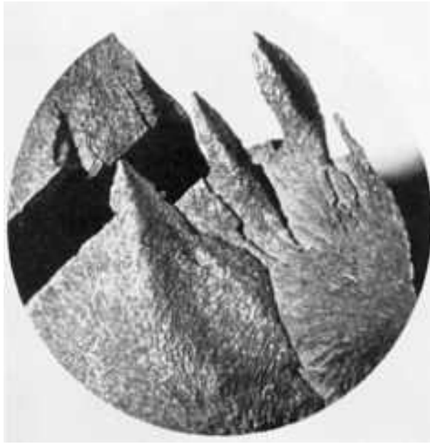
Fig. 768 Surface of an impact fracture in a shear blade of AISI L6 tool steel heat treated to a hardness of 55 HRC. The impact generated the two crack fronts whose junction may be seen at the secondary fissure that enters the field of view at lower right; the radial markings on either side clearly meet this at divergent angles. A third and separate crack front (at top left) met these two crack fronts at the wide secondary crack beneath the projecting shards. 3×
