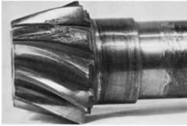
Fig. 510 Bending-fatigue fracture in the heel of one tooth of a spiral bevel pinion of AISI 8617 steel, carburized and hardened to 57 HRC in the case. Fracture resulted from severe pitting. Note that pitting had begun in an adjoining tooth (near top). 0.75×
