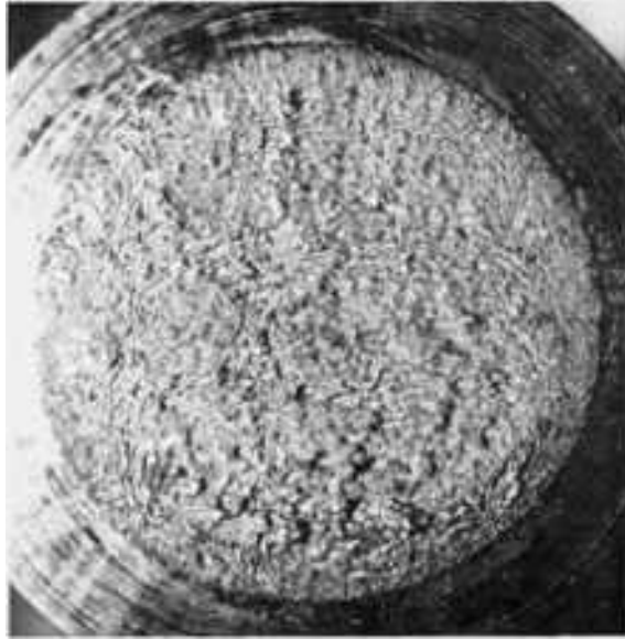
Fig. 429 Tension-overload fracture in a notched specimen similar to those in Fig. 426, 427, and 428, but heat treated to a hardness of 35 HRC. Tested at -40\text{ }^{\circ}\text{C} ( -40\text{ }^{\circ}\text{F} ). The surface shows only fibrous marks. See Fig. 430 and 431 for surfaces of fractures in similar specimens at different test temperatures. 17\times
