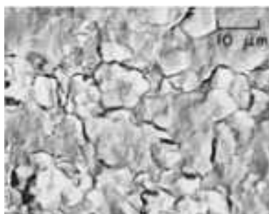
Fig. 1070 TEM p-c replica of the surface of an intergranular fracture in an aircraft landing-gear component of forged aluminum alloy 7075-T6 that fractured as the result of stress-corrosion cracking. Note the secondary cracks between the grains. 1000×
