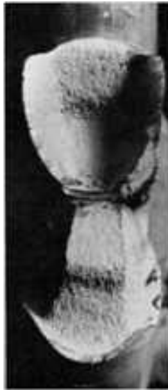
Fig. 455 Matching fracture surfaces of an AISI 4340 steel helicopter bolt that was broken by notch bending. The fine markings are fibrous tear ridges. Note the very large shear lips. 2.5×
