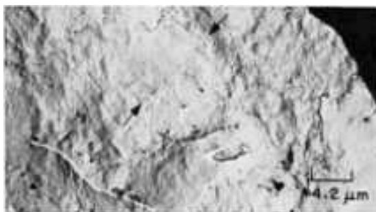
Fig. 842 TEM p-c replica of a fracture surface of one of the turbine-rotor blades in Fig. 840. This view is typical of all the areas examined. A patch of fatigue striations is faintly visible at center between arrows. The fatigue crack is believed to have been initiated by hot corrosion, which was shown, by sectioning of blades, to exist at concentrations of lead. 2400×
