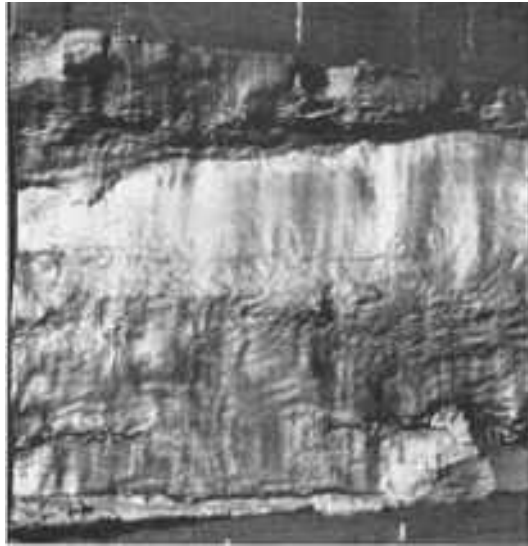
Fig. 770 A "hammer-burst" fracture at the center of a 130-mm ( 5 \frac{1}{8} -in.) diam, 38-mm ( 1 \frac{1}{2} -in.) thick forged disk of AISI T1 tool steel. This longitudinal fracture shows a surface of either a lap or a cold shut; the appearance of such a fracture is often called "platy" or "laminated." 2.3×
