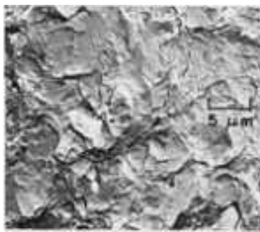
Fig. 461 Surface of a tension-overload fracture in a notched specimen of the same AMS 6434 steel sheet as in Fig. 460, but broken at -73 °C (-99 °F). The dimples here are of the same size and nature as those in Fig. 460. See also Fig. 462. TEM p-c replica, 2000×
