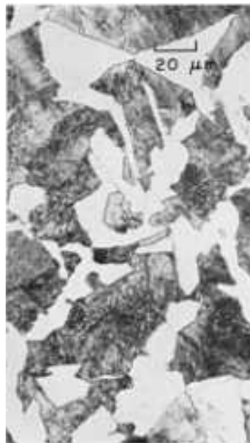
Fig. 178 Polished and etched section through the shell in Fig. 177, showing an as-rolled microstructure consisting of a mixture of ferrite and fine pearlite, which resulted in a maximum hardness of 86 HRB. Nital etch, 500x
