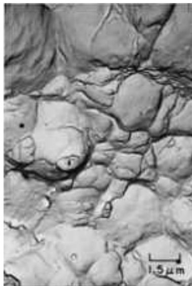
Fig. 709 TEM p-c replica of an area at B in Fig. 704. The equiaxed dimples visible here resulted from tension overload during final fracture, but before final shear rupture. 6500×
