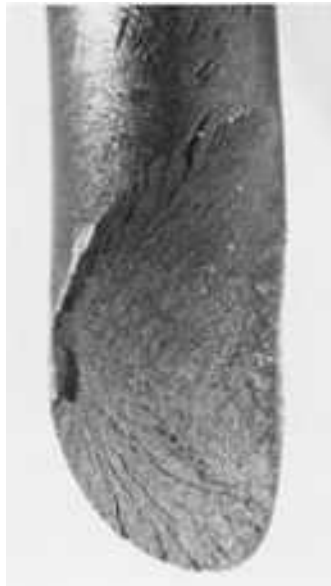
Fig. 266 Fracture surface of the spring in Fig. 265. The crack originated at a screw mark. The small size of the fatigue zone (at left) indicates that final fast fracture occurred soon after crack initiation. 3×
