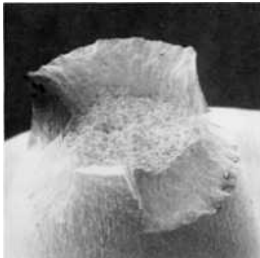
Fig. 798 Surface of a fracture in a tensile-test specimen of 18% Ni, grade 300, maraging steel aged 3 h at 480 °C (900 °F), broken at room temperature. The crack-initiation zone (at center) is an example of extremely uneven fibrous fracture; there appear to be no radial marks leading to the base of the surrounding shear lip. The shear lip is of the pronounced type that is observed when a large reduction in cross-sectional area accompanies fracture. See also Fig. 799, 800, 801, and 802. 26×
