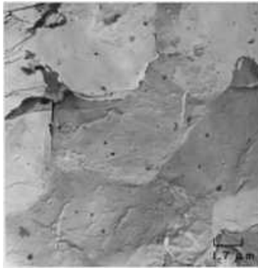
Fig. 409 TEM p-c replica of a region containing the crack-nucleation site near point 2 in Fig. 404. The features that are visible in this region are the same as those in the region shown in Fig. 408, which further indicates that hydrogen embrittlement caused the cracks. 6000×
