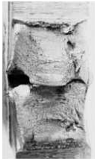
Fig. 1211 Both fracture surfaces of a specimen aged at 700 °C (1290 °F) 2 h and air cooled. Impact energy was about 203 J (150 ft · lb). Much deformation accompanied fracture. See also Fig. 1212. 4.8× (Figures 1207, 1208, 1209, 1210, 1211, 1212, 1213, 1214, 1215, 1216, 1217, and 1218 present six related pairs of light and SEM fractograph of specimens of an Fe-12Ni-0.5Ti alloy intended for use at cryogenic temperatures. The series shows the effect on Charpy impact energy at -196 °C (-321 °F), and on fracture-surface characteristics, of the temperature of aging after austenitizing at 900 °C (1650 °F) for 2 h and air cooling.)
