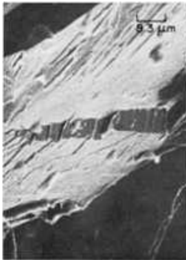
Fig. 1204 Another view of the slow-bending fracture in Fig. 1201, showing a different region of the fracture surface at higher magnification. Here, as in the specimen shown in Fig. 1201 and 1202, fracture was by quasi-cleavage. Also shown is the intersection of a twin boundary with the cleavage plane. See also Fig. 1205. SEM, 1200×
