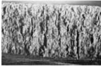
Fig. 22 A companion notch-impact fracture to the one shown in Fig. 21, but here the longitudinal stringers of slag are normal to the fracture surface. Individual particles of slag are not readily visible at this magnification, but they cause the speckled appearance. 6×
