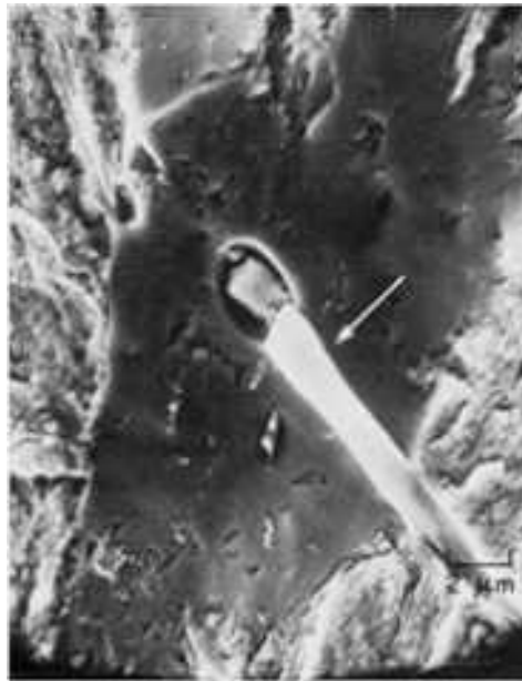
Fig. 388 View, at still higher magnification, of the inclusion in Fig. 386 and 387, showing that the inclusion was fractured by cleavage. The cleavage surface bears a bright metal silver (at arrow). SEM, 5000×
