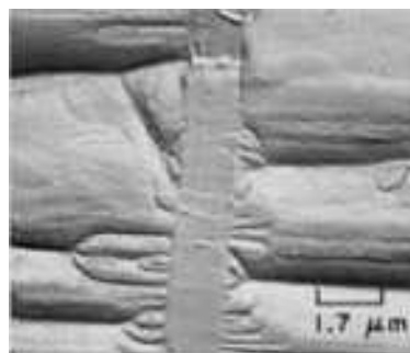
Fig. 1178 Fracture produced by tension over-load in a specimen of titanium alloy Ti-7Al-2Nb-1Ta, showing staining and very large dimples. Vertical band at center is where crack initiated at a second-phase region and propagated to left and right. TEM p-c replica, 6000×
