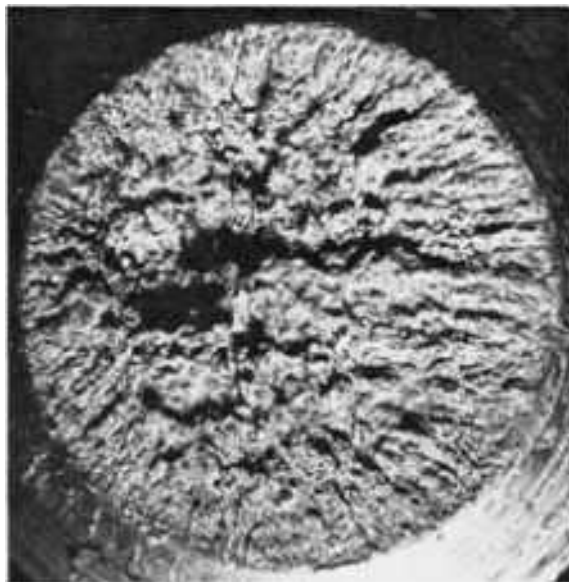
Fig. 428 Surface of tension-overload fracture in a third notched specimen of AISI 4340 steel, the same as those in Fig. 426 and 427, but tested at 155\text{ }^{\circ}\text{C} ( -245\text{ }^{\circ}\text{F} ). At this low test temperature, a completely radial fracture was produced. The surface shows no fibrous zone, only radial marks. 17\times
