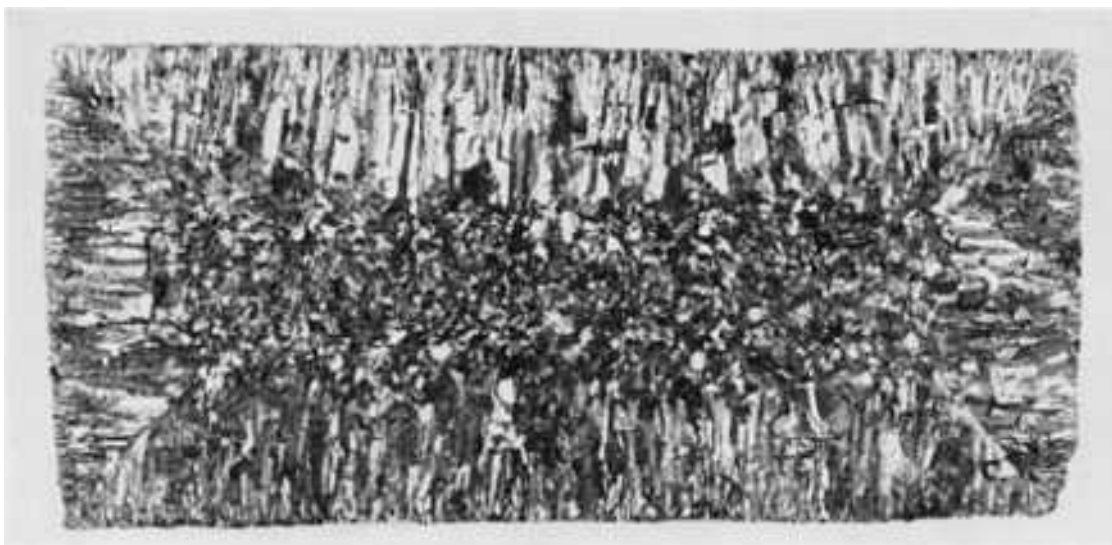
Fig. 109 Fracture surface of a small ingot of iron-chromium-aluminum alloy. The as-cast solidification pattern is clearly revealed. 0.57×
