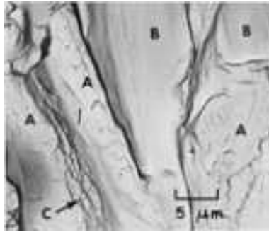
Fig. 1176 Bending fracture in a specimen of titanium alloy Ti-6Al-4V that broke by stress-corrosion cracking in 3.5% NaCl (areas A), but that also exhibits regions of stretching (areas B) and a step containing what appear to be dimples (arrow at C). TEM p-c replica, 2000×
