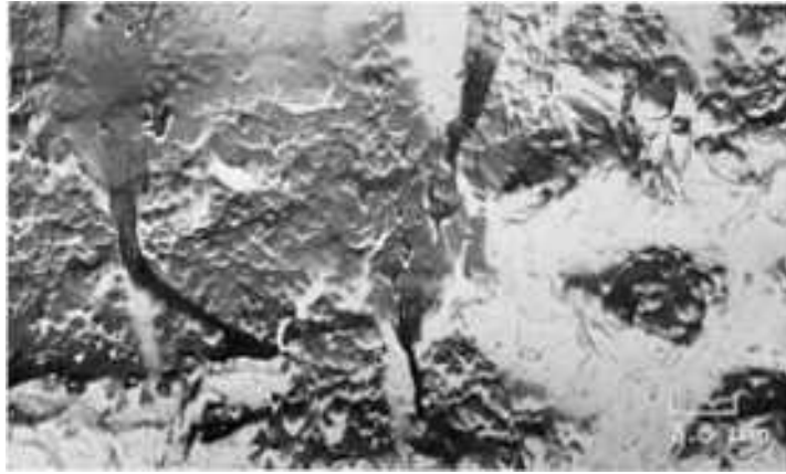
Fig. 393 Surface of a fracture in a specimen of AISI 4340 steel that was broken by impact at room temperature, showing small dimples of quite uniform size, some of which (at right) are equiaxed. At left are elongated tear dimples pointing toward a tear ridge (at bottom). At upper left are regions in which considerable local stretching has occurred. Some secondary cracking may be present. TEM p-c replica, 3000×
