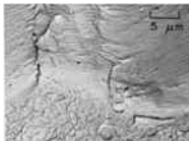
Fig. 1071 TEM p-c replica of the surface of a fracture in a specimen of aluminum alloy 7075-T6 that first was
