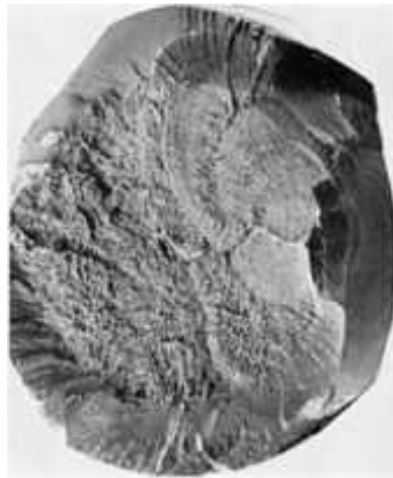
Fig. 198 Surface of a fatigue fracture in a truck axle of AISI 1041 steel induction hardened to 55 HRC. The axle broke after 490 h of service. Crack origin was subsurface, near a keyway. Note that fatigue crack progressed in steps. Actual size.
