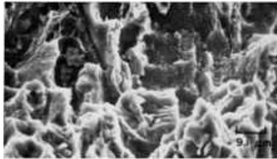
Fig. 1010 A portion of the tension-overload fracture surface in Fig. 1009, as seen at ten times the magnification there, which reveals fine details. A number of medium-size dimples contain inclusions, some of which are broken. In contrast are the minute dimples visible at left and right in the upper portion of this view. SEM, 1100 \times
