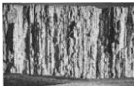
Fig. 20 Fe, 0.01% C, 0.24% Mn, and 0.02% Si, heat treated at 950 °C (1740 °F) \frac{1}{2} h, air cooled. The structure is ferrite. Hardness, 62 HV. The fracture was generated by impact at -196 °C (-321 °F). Cleavage steps beginning at the twin at top form a sharply defined river pattern. Crack propagation was in direction of arrow. SEM, 300×
