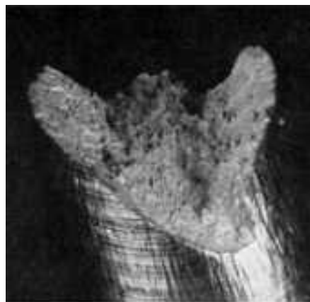
Fig. 1015 Surface of a tension-overload fracture in an unnotched specimen of aluminum alloy 7075-T6 having a tensile strength of 520 MPa (75 ksi), with 22% reduction of area. Surface is coarsely fibrous; shear lip has formed two opposing lobes. See also Fig. 1016 and 1017. 9×
