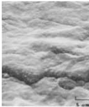
Fig. 33 Stress-corrosion fracture that occurred by decohesion along the parting plane of an aluminum alloy forging
