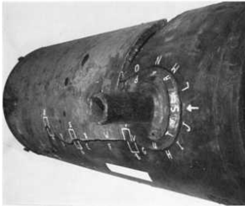
Fig. 177 Fractured shell of an 865-mm (34-in.) diam pressure vessel fabricated from a 32 by 2440 by 9145 mm ( 1\frac{1}{4} by 96 by 360 in.) plate of ASTM A515, grade 70, steel for pressure vessels. The shell broke during testing at an internal gage pressure of 8.3 MPa (1.2 ksi). The fracture, which originated adjacent to a flange (arrow at S), followed a very complex path. See also Fig. 178, 179, 180, 181, 182, 183, 184, 185, and 186. ~0.17x
