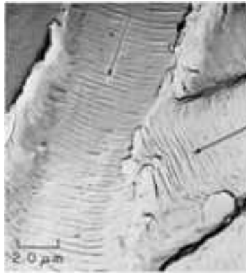
Fig. 27 Striations on two joining, independent fatigue crack fronts on a fracture surface of aluminum alloy 6061-T6. The two arrows indicate direction of local crack propagation. TEM p-c replica
