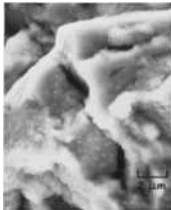
Fig. 737 Enlargement of the area in the rectangle in Fig. 736. The oxide coating appears to be quite continuous, except for the scattered secondary cracks. Compare with Fig. 738. SEM, 5000×
