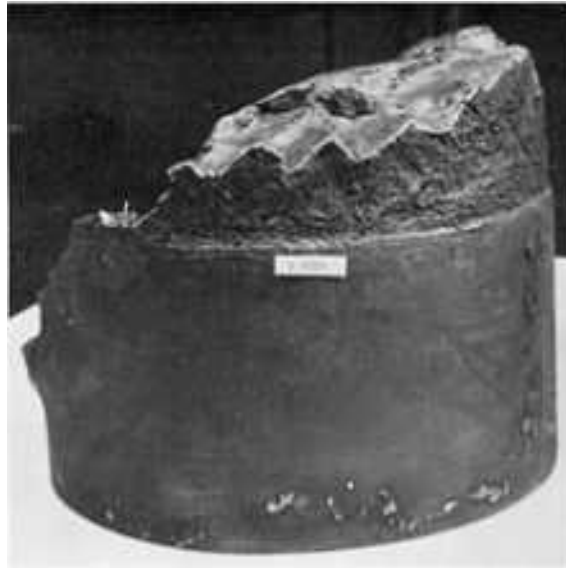
Fig. 153 Side view of the fractured drive shaft in Fig. 152. Note the serrated profile (retouched for clarity) of this edge of the fracture surface and the diagonal cracks on the shaft surface. The cracks were caused by corrosion fatigue from the combination of reversed shaft torsion, perhaps some bending, and seawater attack. 0.8x
