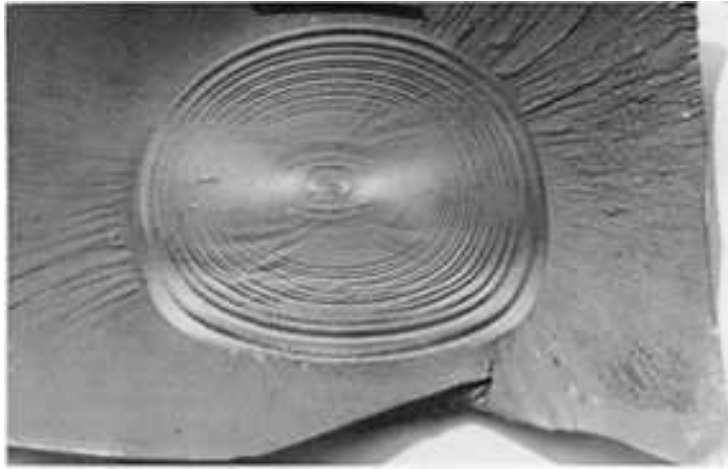
Fig. 55 Circular spall that began at a large subsurface inclusion in a hardened steel roll
