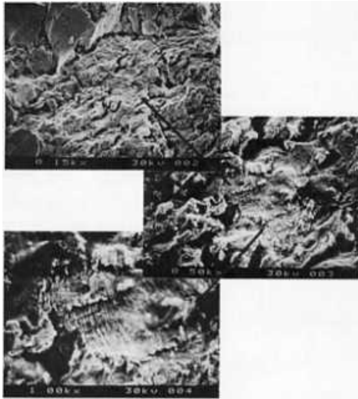
Fig. 17 Poorly defined fatigue striations in a low-carbon steel specimen
