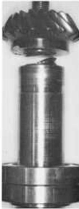
Fig. 342 Fatigue fracture in an AISI 4140 steel tail-rotor drive-pinion shaft of a helicopter, heat treated to a hardness of 35 HRC. See also Fig. 343, 344, 345, and 346. Actual size
