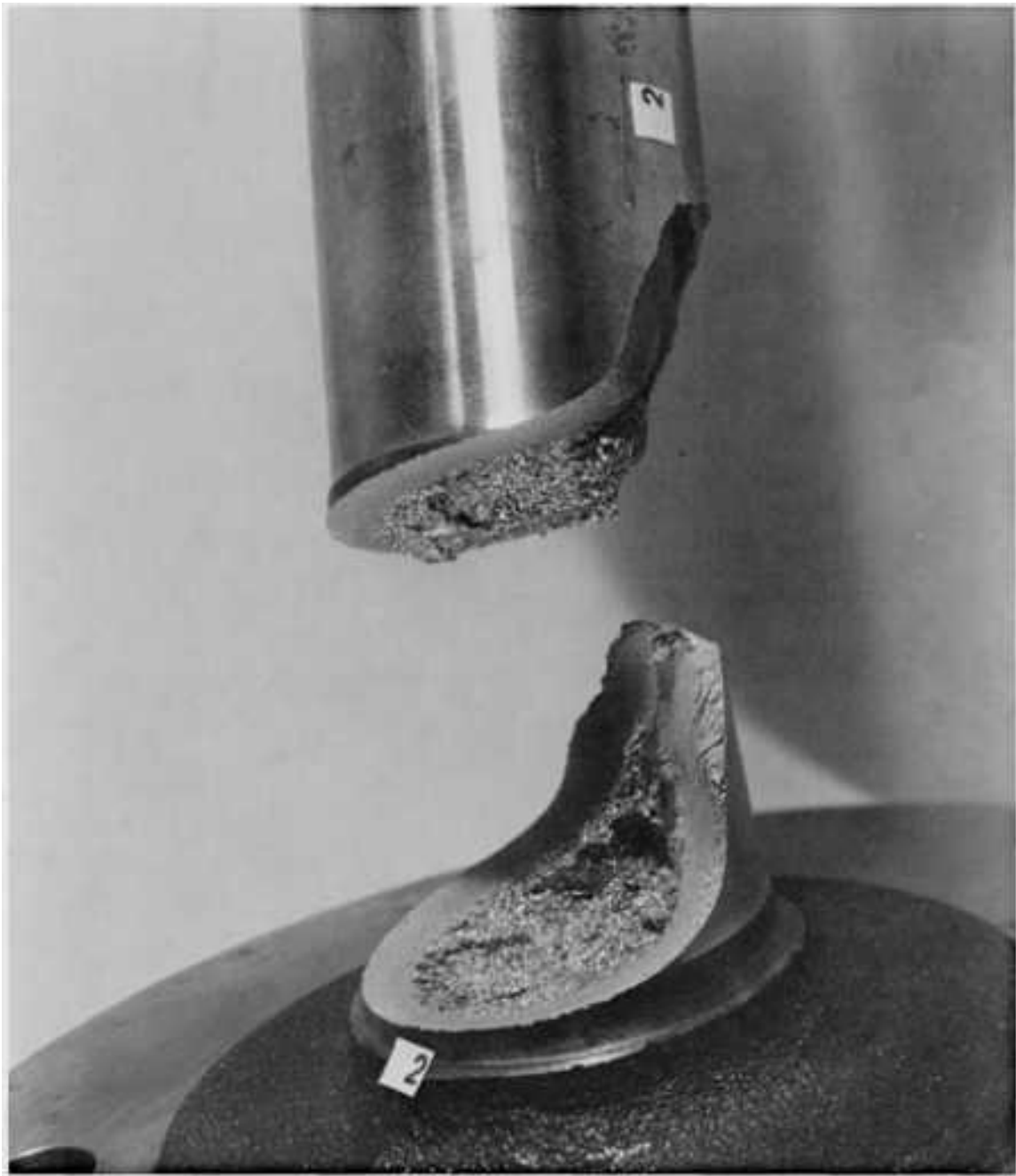
Fig. 221 Brittle fracture of a modified SAE 1050 axle shaft due to single bending impact load. Steel nominal composition: 0.50% C, 0.95% Mn, 0.25% Si, 0.01% S, and 0.01% P. The hot-rolled and upset shaft had an induction-hardened martensitic case (60 HRC) and a pearlite-ferrite core (20 HRC). Failure occurred at the flange end. Part was broken in the laboratory. Shown in this fractograph are the fracture surfaces, including a compression chip. See also Fig. 220, 222, 223, 224, 225, 226, and 227. Actual size (General Motors Research Laboratories)
