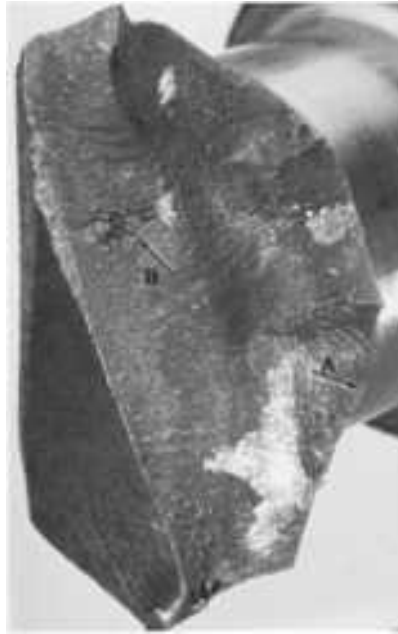
Fig. 41 Surface of a fatigue-test fracture in an experimental crankshaft of induction-hardened 80-60-03 ductile iron with a hardness of 197 to 225 HB. Fatigue-crack origin is at arrow A. Porosity at arrow B was unrelated to fracture initiation. 2.5×
