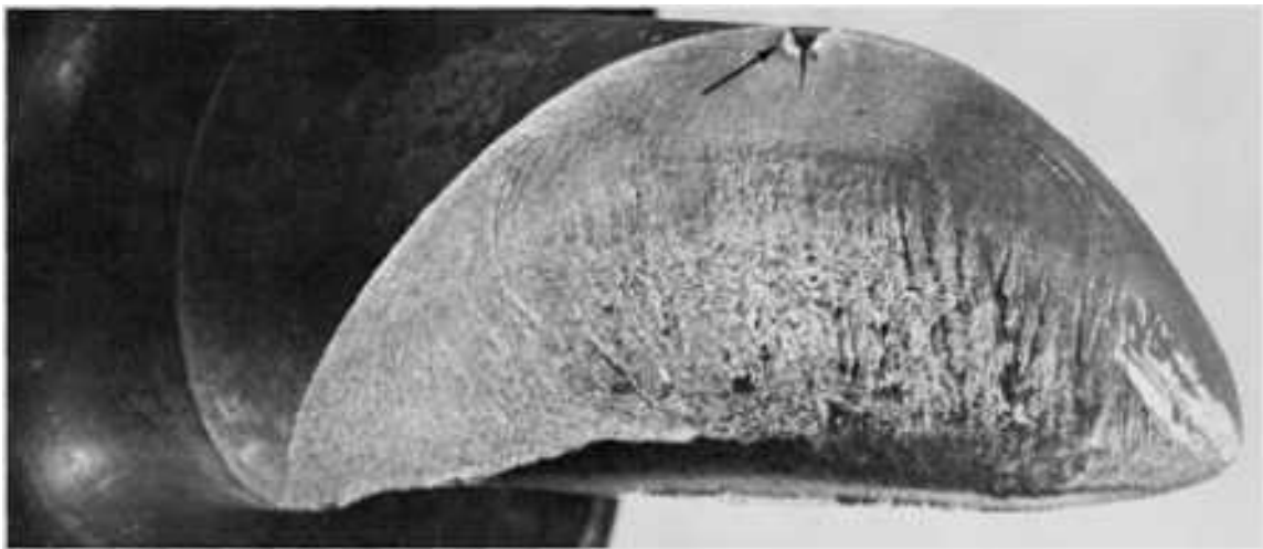
Fig. 234 Surface of a fatigue fracture in a full-floating axle of an AISI 1050 steel induction hardened to about 50 HRC. The axle was tested in reversed torsion. The arrow indicates the origin of the fatigue crack, which grew by shear fatigue to the small, circular beach mark. Subsequent crack growth was by tension fatigue until final fracture (brittle tensile) occurred under a single torsional load. \sim 2\times
