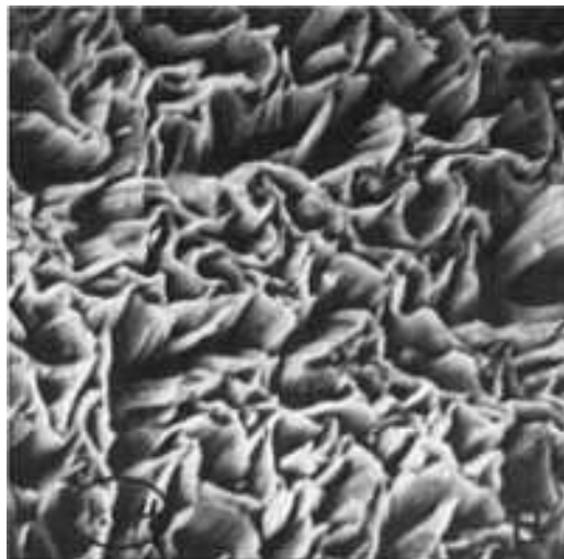
Fig. 1272 Higher-magnification view of an area of tungsten fiber P in Fig. 1271. Deformation during fracture has thinned the walls of the dimples to sharp edges, which shows the highly ductile nature of the fracture. Note the uniformity in height of the walls. Compare with Fig. 1262. SEM, 10,000×
