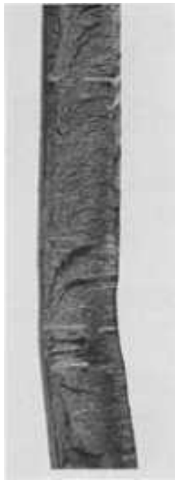
Fig. 111 Example of inclusion stringers (white streaks against the dark background) on a longitudinal test fracture. The specimen was blued to reveal the stringers.
