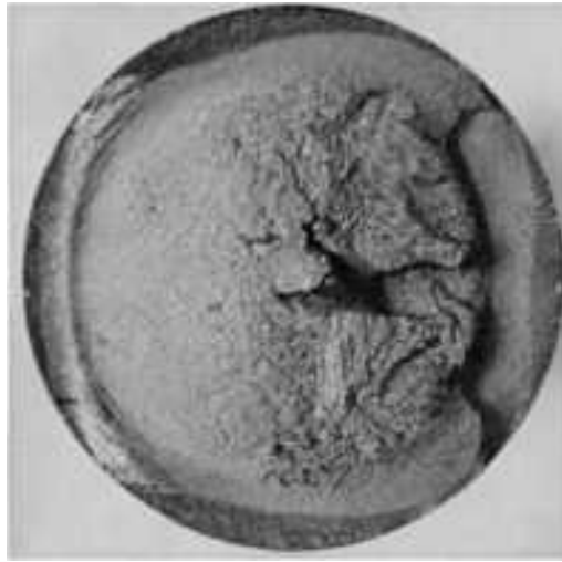
Fig. 201 Fatigue-fracture surface of a case-hardened AISI 1039 steel shaft. Case hardness, 50 HRC; core, 19 HRC. Note that fracture of the case was nearly complete before the fatigue cracks penetrated into the core. 2×
