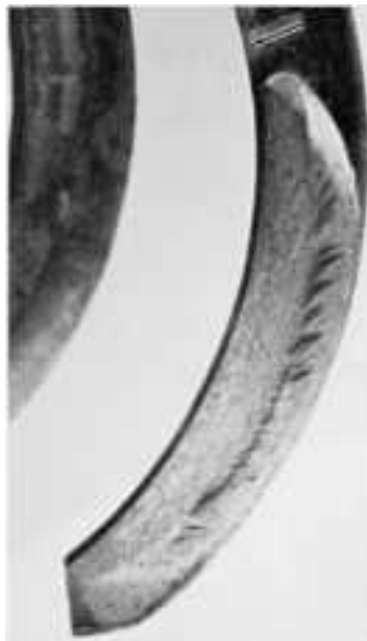
Fig. 261 Fatigue-fracture surface of a suspension spring of AISI 10B62 steel wire with a hardness of 460 HB. Note the fine seam (at arrow), which is the fatigue-crack origin. 2\times
