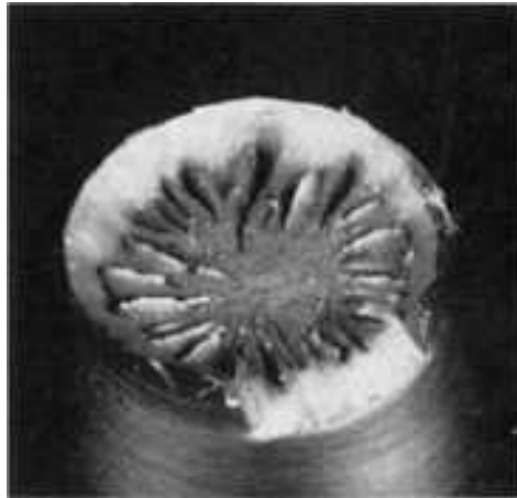
Fig. 530 Tensile-overload fracture in an unnotched specimen of AISI 8740 steel; tensile strength, 1351 MPa (196 ksi). A cup-and-cone fracture with a fibrous zone containing radial features between the central fibrous region and the shear lip. See also Fig. 531 and 532. 9×
