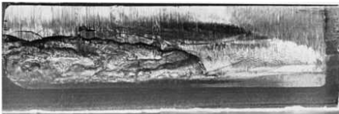
Fig. 512 Surface of a spalling-fatigue fracture in a single tooth of a heavily loaded final-drive pinion of AISI 8620 steel, carburized and hardened to 60 HRC in the case, showing vertical scratches, which indicate that appreciable abrasive wear took place also. The surface ripples at right suggest that a small amount of plastic flow occurred under the applied load. ~4×
