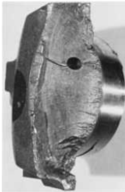
Fig. 42 Surface of a fatigue-test fracture in an experimental crankshaft of ductile-iron with a hardness of 241 to 255 HB. Note the multiple fatigue-crack origins at the journal edge (at right). Fatigue beach marks are evident, which is unusual in cast iron. Actual size
