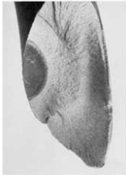
Fig. 264 Fatigue fracture in a 16-mm ( \frac{5}{8} -in.) diam suspension spring of AISI 10B62 steel wire. The fatigue crack probably originated at a surface defect and grew so slowly that oxidation occurred (note darkness of fatigue zone at left). 3×
