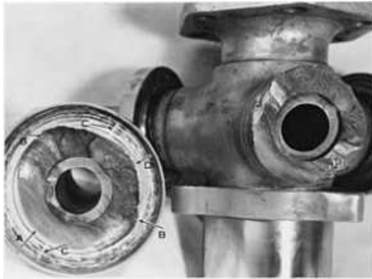
Fig. 451 Mating surfaces of a fatigue fracture in a blade arm of a forged aircraft propeller-hub spider of AISI 4340 steel and through the central pilot tube of the arm. The fatigue crack originated in the fillet between the bearing-retention flange and the blade arm. Hardness of the forging was 35 HRC. The origin is at arrow A (lower left), at an inclusion. The fatigue crack penetrated as far as the locations indicated by arrows B before final fast fracture occurred. Alignment of the bearing-race parting line (arrows C) was not as specified. Arrow D indicates the region of final fast fracture. See Fig. 452 for a higher magnification view of this region. 0.6×
