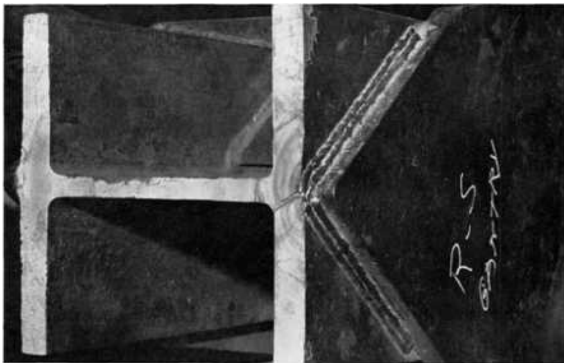
Fig. 207 Surface of a fatigue fracture in a medium-carbon steel I-beam, with a flange 400 by 400 by 40 mm
