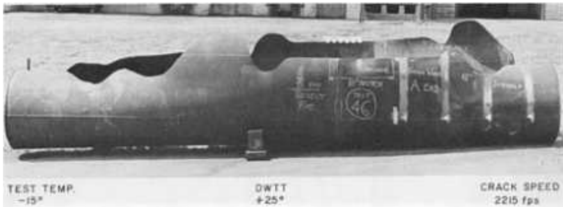
Fig. 46 Fracture of API grade X-60 line pipe tested 22 °C (40 °F) below the 50% shear area drop-weight tear test transition temperature. Temperature given in °F. See also Fig. 42, 43, 44, and 45.
