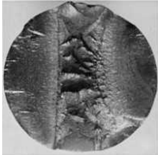
Fig. 202 Surface of a fatigue fracture in a shaft of AISI 1041 steel with a hardness of 302 HB. The shaft was broken by reversed stressing. Note the two fatigue-crack origins at right edge and the third origin at left. 2×
