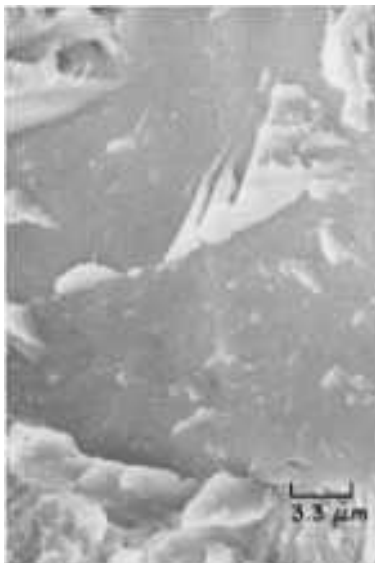
Fig. 569 Higher-magnification view of the area in the rectangle in Fig. 568. A tongue-like formation is visible (at left center) on the flat surface of a grain. Tempering has produced embrittling networks of carbide particles. SEM, 3000×
