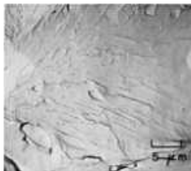
Fig. 27 Cleavage fracture in Armco iron broken at -45 °C (-49 °F). Instead of cleavage steps, tear ridges (occasionally forming river patterns) were produced here by microscopic plastic flow. TEM p-c replica, 2000×
