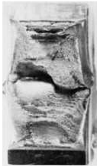
Fig. 1213 Both fracture surfaces of a specimen aged at 750 °C (1380 °F) 2 h and air cooled. Impact energy was about 203 J (150 ft · lb); deformation is similar to that in Fig. 1211. See also Fig. 1214. 4.8× (Figures 1207, 1208, 1209, 1210, 1211, 1212, 1213, 1214, 1215, 1216, 1217, and 1218 present six related pairs of light and SEM fractograph of specimens of an Fe-12Ni-0.5Ti alloy intended for use at cryogenic temperatures. The series shows the effect on Charpy impact energy at -196 °C (-321 °F), and on fracture-surface characteristics, of the temperature of aging after austenitizing at 900 °C (1650 °F) for 2 h and air cooling.)
