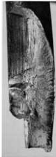
Fig. 259 Fatigue fracture in AISI 1060 steel spring wire, 4.6-mm (0.18-in) diam, originating at two or more crack nuclei at and above lower shoulder at left edge. 7×
