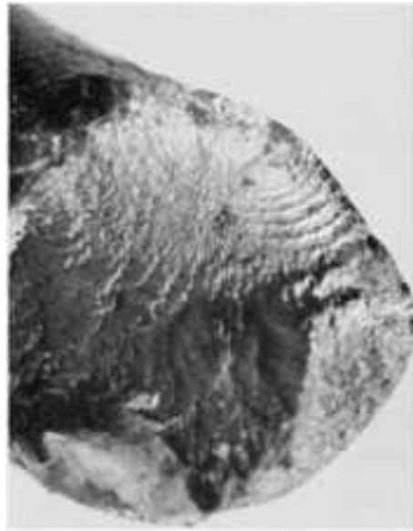
Fig. 270 Fracture surface of spring at right side in Fig. 269, shown at higher magnification. The nucleus of the fatigue crack is clearly visible on the wire surface at top, with a succession of beach marks fanning out below it. The surface of the zone of final fast fracture appears to be quite woody. 15×
