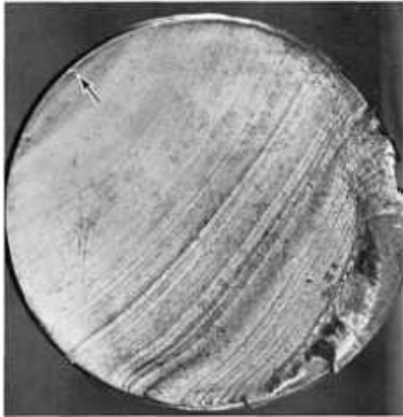
Fig. 522 Surface of a fatigue fracture in a nonrotating axle of AISI 8640 steel with a hardness of approximately 30 HRC. Visible are beach marks, which indicate that the fatigue crack penetrated across more than 90% of the axle before final fast fracture occurred. The origin (arrow) was at a discontinuity in a cut thread. \sim 0.95\times
