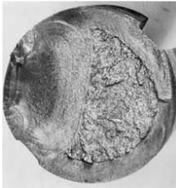
Fig. 200 Surface of a fatigue fracture in a keyed axle of AISI 1041 steel induction hardened to 50 HRC. An accidental arc strike on the axle surface, at left, initiated a fatigue crack, which grew about halfway through the cross section before fast fracture occurred in the hardened zone; fast fracture progressed from both sides of the fatigue crack, as shown by chevron marks. 1.3×
