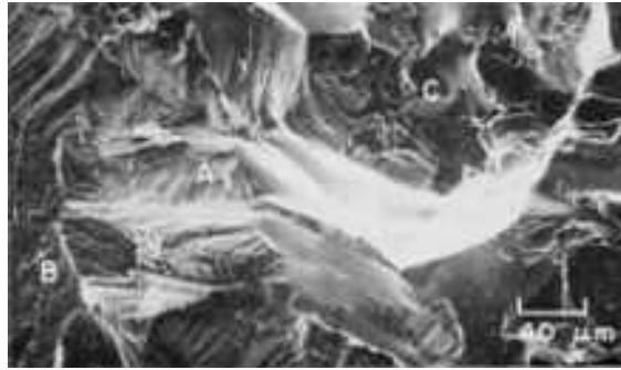
Fig. 1052 Fatigue-fracture surface of a test bar cast from aluminum alloy 7075, aged to the T6 temper and then tested in a 3.5% NaCl solution. A diagonal region of fatigue striations is visible at A; this region abuts areas of intergranular fracture (at B) and interdendritic porosity (at C). SEM, 250×
