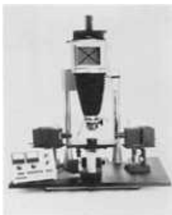
Fig. 5 View camera with a scanning light photomacrography system. Courtesy of Irvine Optical Corporation.
