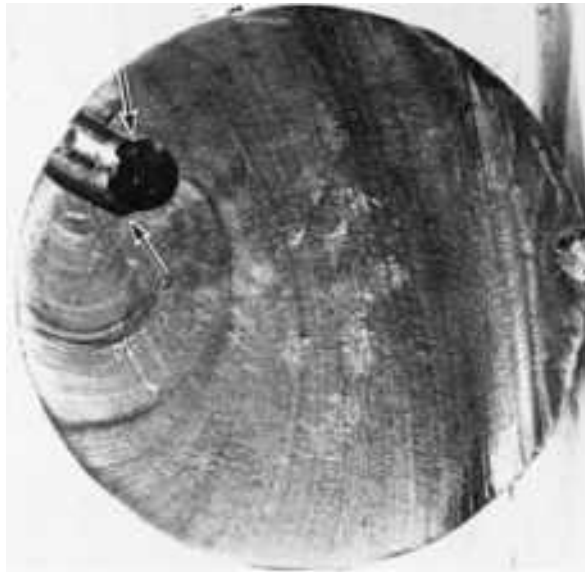
Fig. 520 Surface of a fracture in an AISI 8640 boom-point pin that broke during service. Steel was quenched and then tempered to a hardness of 269 HB. Sharp corners of mismatched transverse grease holes provided stress concentrations that generated two fatigue cracks (arrows). Actual size.
