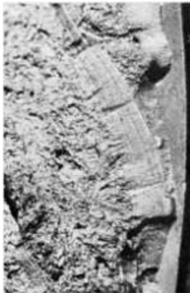
Fig. 452 View of an area at arrow D in Fig. 451, in the region of final fast fracture. Fatigue patches are interspersed among areas of rapid crack advance, indicating that final fracture occurred in stages. 10×
