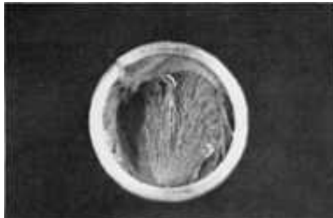
Fig. 732 Surface of a fracture in a threaded specimen of 13-8 PH stainless steel (same properties as for the specimen in Fig. 726) that was heavily charged with hydrogen by plating without subsequent baking. The specimen broke during loading. The crack origin, visible at bottom edge, grew both circumferentially and radially. See also Fig. 733. 6×
