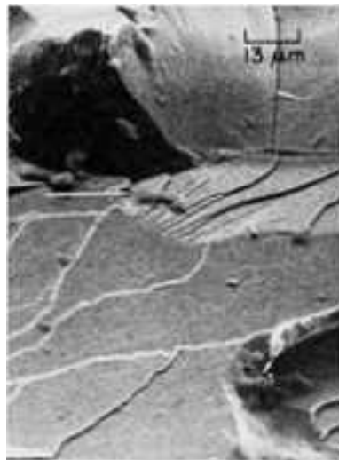
Fig. 1205 Surface of a bending fracture in a specimen of the same alloy and the same history as that in Fig. 1203, showing assorted river patterns. Note twist boundary at center, which has generated several cleavage steps. Although the higher nickel content of the alloy in Fig. 1201 gave greater strength, the aspects of subzero impact rupture are about the same for both alloys. See also Fig. 1206. SEM, 750×
