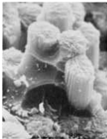
Fig. 1308 Fracture surface of a longitudinal (0°) carbon/epoxy specimen that failed in tension. Specimen was tested at 25 °C (77 °F) in the dry condition. This fractograph shows typical tensile failure of the epoxy resin in a local resin-rich region. This results when fibers break and produce overload tensile failure in the resin. SEM (same conditions as in Fig. 1294), 2000× (The composite specimens shown in Fig. 1296, 1297, 1298, 1299, 1300, 1301, 1302, 1303, 1304, 1305, 1306, 1307, 1308, 1309, and 1310 all consisted of circa 1978 Thornel 300 fibers in Narmco 5208 epoxy resin. The composites were all fabricated by lay-up of prepreg tape and were autoclave cured 175 °C (350 °F) according to the manufacturer's recommendations. Specimens were then end-tabbed and cut in accordance with the ASTM D3039. The 0° and 90° tensile specimens were tested in
