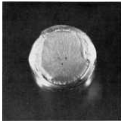
Fig. 1168 Fracture surface of a specimen of titanium alloy Ti-6Al-4V (same mechanical properties as in Fig. 1162) broken in low-cycle fatigue (26,000 cycles) in tension-tension ( R = 0.1 ) at maximum loading of 689 MPa (100 ksi). Several crack origins are visible at bottom. See also Fig. 1169. 6×
