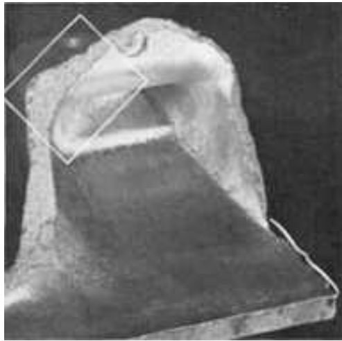
Fig. 921 A portion of a fractured carrier tray and sand cast of an aluminum alloy intended to be 356.0-T6. Chemical analysis revealed that the copper and zinc contents were of an order of magnitude above the specified limits. The silicon content was approximately as dictated by the specification. The hardness measured 82 HB--appreciably above the 70 HB expected. Tensile strength was 179 to 193 MPa (26 to 28 ksi)--slightly below the specified minimum of 207 MPa (30 ksi). See Fig. 922 for the area in the rectangle and Fig. 923 for bracketed area at a magnification of 3×. Actual size
