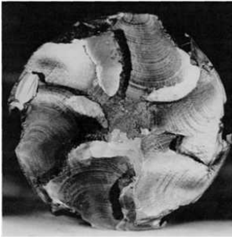
Fig. 473 Rotating bending fatigue fracture of an AISI 4817 shaft, carburized and hardened to 60 HRC on the surface. Fracture initiated in six fillet areas around the periphery, near the runouts of six grooves. Each fatigue area propagated separately, but uniformly, inward to final rupture at the center. Cause of fracture was traced to grinding damage in the fillet. The bright and shiny flat areas are regions of postfracture damage produced by the rubbing together of the broken portions of the shaft. (D.J. Wulpi, Consultant)
