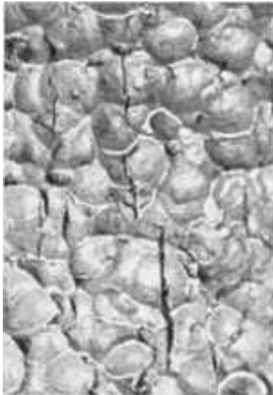
Fig. 993 Surface of the shot-peened fillet of another companion propeller blade to that in Fig. 990, showing the same type of fatigue cracks as those in the propeller blade shown in Fig. 992. These cracks were present in large numbers in the fillet area. 20×
