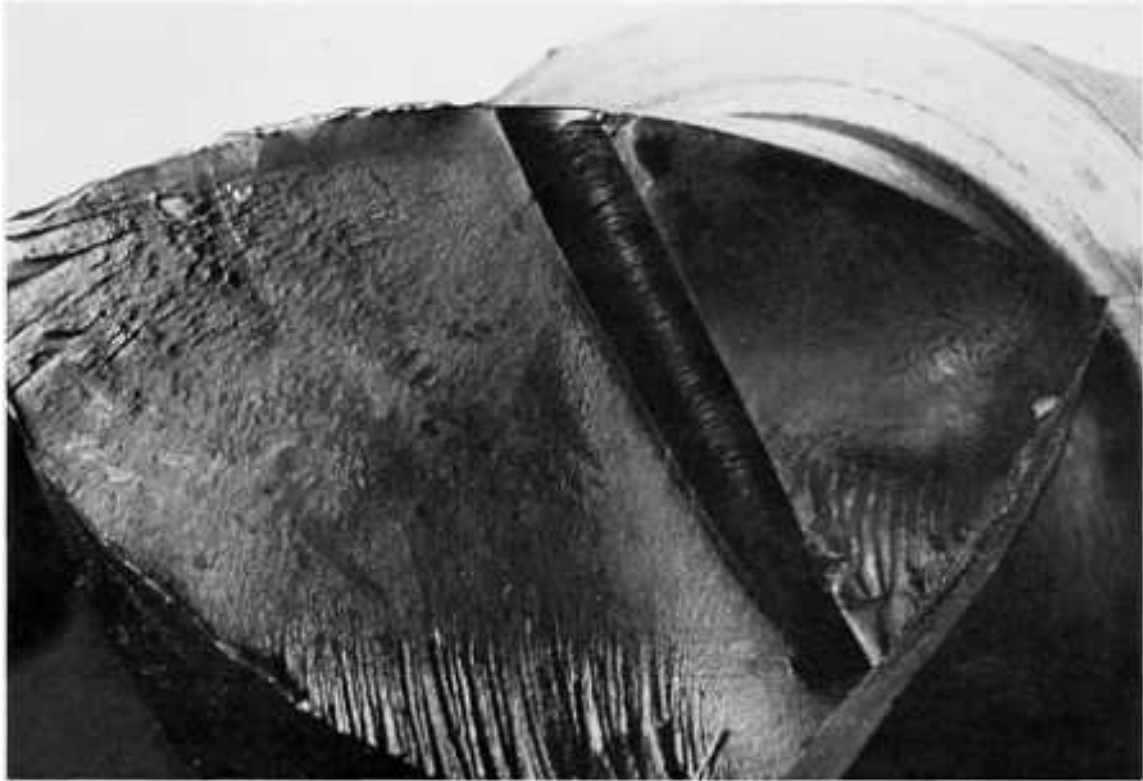
Fig. 216 Surface of a torsional-fatigue fracture in an AISI 1045 steel crankshaft induction hardened to 55 HRC. The crack originated at the edge of an oil hole. Although it is not clearly evident in this view, the crack grew at a 45° angle to the axis of the crankshaft because of tensile-stress components caused by the torsional loading. 2.5×
