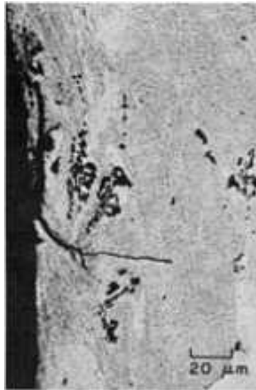
Fig. 995 Another polished and etched section through the shot-peened fillet of the fractured blade in Fig. 990, showing a fatigue crack that grew from a surface flaw. The structure indicates that only very superficial shot-peening occurred here. Etched in Keller's reagent, 500×
