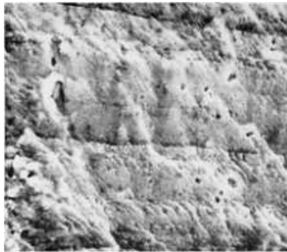
Fig. 980 Fatigue fracture of an aluminum alloy 2014-T6 heat-treated forging. Details of the heat-treatment procedure were not available. Some machining was carried out on the forging prior to heat treatment. The aircraft structural component cracked in service. The horizontal lines on the fracture surface are grain boundaries. Fatigue striations are also visible, traversing the fracture face at roughly 60°. Note the absence of discontinuities at their intersections with the grain boundaries. SEM, 1800× (E. Neub, University of Toronto)
