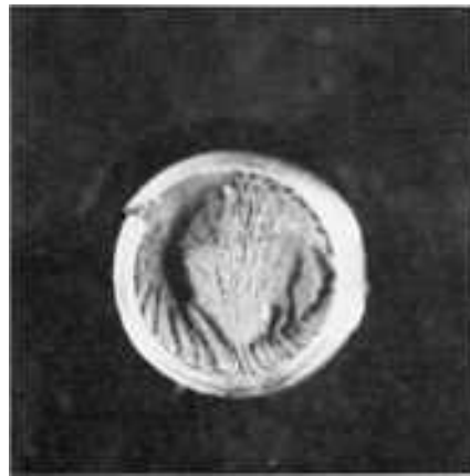
Fig. 789 Fracture caused by hydrogen embrittlement in threaded specimen of AISI H11 tool steel (same heat treatment and tensile strength as in Fig. 786). Hydrogen impregnation was by plating. Fracture occurred before the full sustained load could be applied and progressed around the circumference of the specimen. See also Fig. 790 and 791. 6×
