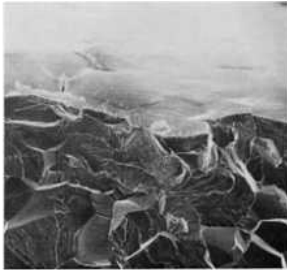
Fig. 1089 The external surface (top) and the corrosion-fatigue fracture surface (bottom) of a solution-treated and peak-aged Al-5.6Zn-1.9Mg sample tested in high-purity deaerated water. SEM, 100× (R.E. Ricker, University of Notre Dame, and D.J. Duquette, Rensselaer Polytechnic Institute)
