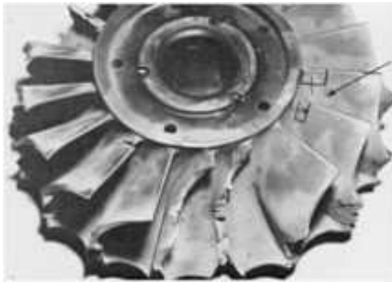
Fig. 839 A gas-producer turbine rotor cast of alloy 713LC that fractured after 440 h of service, as the result of hot corrosion fatigue. Fracture was abrupt, with three blades being thrown off. See Fig. 841 for a view of the area near the arrow. See also Fig. 840 and 842. 0.5×
