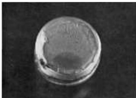
Fig. 729 High-cycle fatigue fracture in threaded specimen of 13-8 PH stainless steel (same properties as for specimen in Fig. 726) tested in tension-tension ( R = 0.1 ) with maximum loading at 30% of tensile strength. Fracture occurred at 959,000 cycles. Note the crescent-shaped crack nucleus. See also Fig. 730 and 731. 6×
