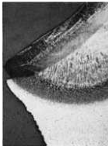
Fig. 180 Polished and etched section through the toe of the flange weld at S (crack nucleus) in Fig. 179, taken normal to the fracture surface (at left). The toe of the weld had a maximum hardness of 45 HRC. Nital etch, 6×
