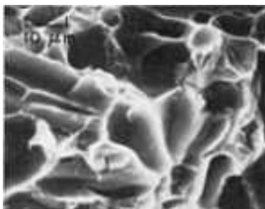
Fig. 946 Higher-magnification view of the area in the rectangle in Fig. 945. Although the features here strongly resemble those shown in Fig. 942, close scrutiny reveals the presence of tiny dimples in the edges of some cells. SEM, 1000×
