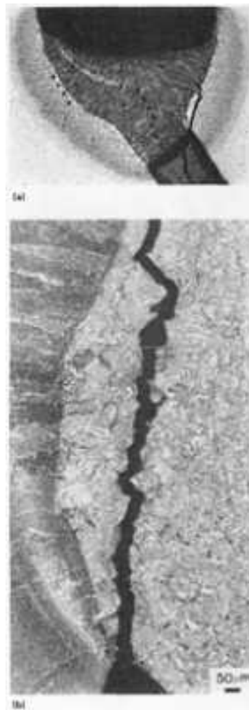
Fig. 108 Stress-relief crack in plate steel Lehigh restraint sample. The crack is intergranular, but the high restraint level suppresses crack branching. The square marks in the weld HAZ in (a) are hardness impressions. (a) 9 \times . (b) Etched with 2% nital. 74 \times
