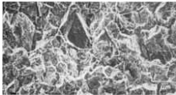
Fig. 905 Fracture surface of a fully aged fracture-toughness test specimen of Cu-2.5Be similar to that in Fig. 904, but aged 3 h at 315 °C (600 °F) before being tested in air. Tensile strength was 1240 MPa (180 ksi). The dimples on the transgranular facets are much finer than in Fig. 904, and there is a network of secondary cracks that appear to be intergranular. One facet (at top center) appears to have formed by quasi-cleavage. SEM, 600×
