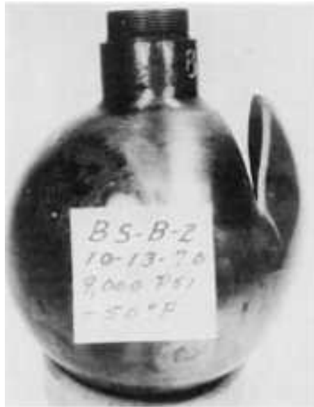
Fig. 20 Macrograph showing ductile overload fracture of a high-pressure steel vessel tested at -45^{\circ}\text{C} ( -50^{\circ}\text{F} ). See also Fig. 19.
