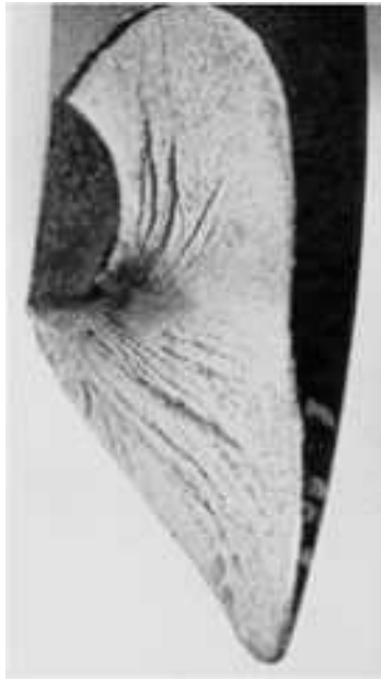
Fig. 260 Surface of a fatigue fracture in 16-mm ( \frac{5}{8} -in) diam spring wire of AISI 1060 steel. The crack origin, which undoubtedly was a surface flaw, generated a fatigue zone (dark area at upper left). The fatigue crack grew slowly, and beach marks became obscured by oxide. \sim 3\times
