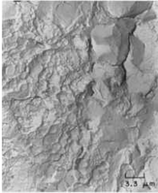
Fig. 407 TEM p-c replica of a region near the right edge of the fracture surface in Fig. 405, showing a transition from intergranular facets (at right) to dimples (at left). This transition is typical of all cracks in the actuator shaft that originated near holes, in each instance, transition occurred at 0.5 to 1.8 mm (0.02 to 0.07 in.) from the edge of the hole. 3000×
