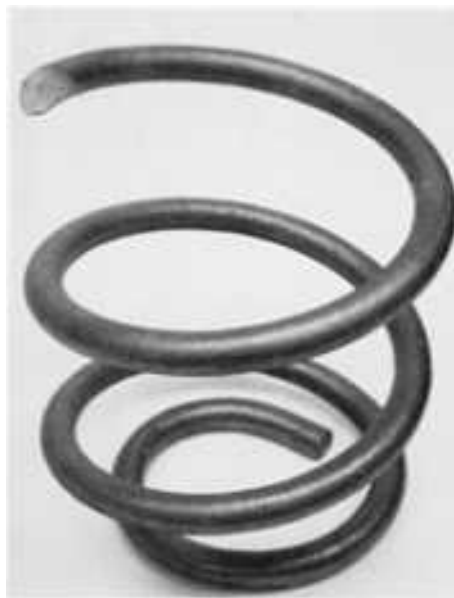
Fig. 267 Fatigue-fractured spring formed from 16-mm ( \frac{5}{8} -in.) diam AISI 1060 steel wire. The seam on the back side of the top turn enters the fracture surface at the dark spot at left edge. See Fig. 268 for a view of the fracture surface. 0.5×
