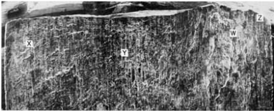
Fig. 1037 Composite of three low-magnification SEM fractographs of the surface of the fatigue fracture at A in Fig. 1035 after ultrasonic cleaning. A small portion of the attachment hole is visible along the top of this view. The lack of beach marks here is perhaps due to the brevity of the test (25 h). Attempts to locate the exact point of crack initiation were not successful, because of the presence of tool marks at the edge of the attachment hole. It is believed, from the orientation of the fatigue striations at W, X, Y, and Z (see Fig. 1038, 1039, 1040, and 1041 for enlarged views of these areas), that the crack began at top right, near the edge of the attachment hole. 26×
