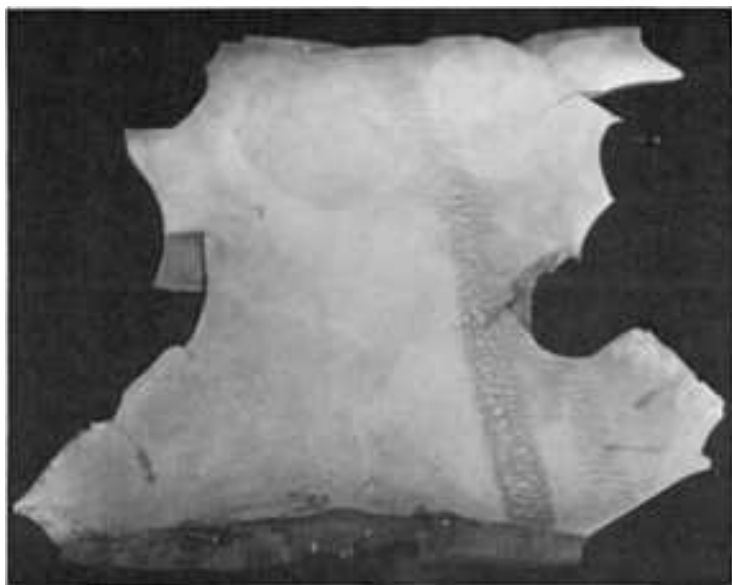
Fig. 66 The roll surface of the spall shown in Fig. 65 after macroetching with 10% aqueous \text{HNO}_3 . Etching revealed a craze crack pattern similar to heat checks, caused by abusive service conditions. About 0.5×
