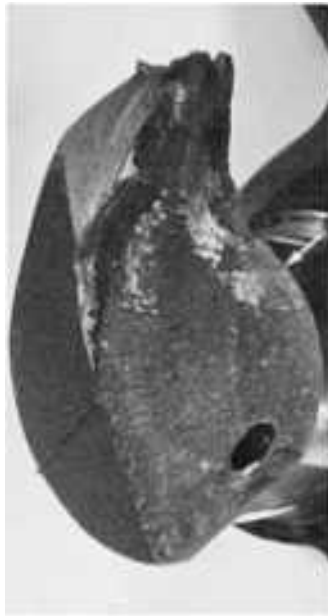
Fig. 43 Surface of a fatigue fracture in an experimental crankshaft broken in a fatigue test. The material is ductile iron with a hardness of 241 HB. The origin of the fatigue crack is at the edge of the journal, at arrow. Actual size
