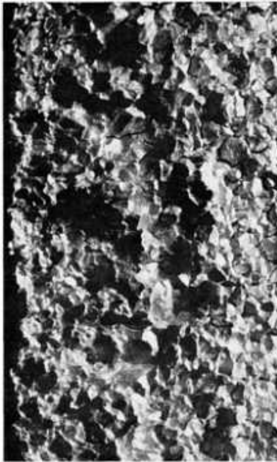
Fig. 615 Higher-magnification view of fracture surface in Fig. 614. This bloom fractured during rolling, splitting apart and wrapping itself around the roll. Note lack of deformation of grains. The fracture surface was cleaned with \text{H}_2\text{SO}_4 and was brightened with a solution containing \text{HNO}_3 and HF. 1.5×
