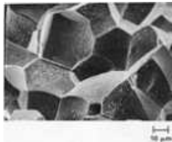
Fig. 58 Corrosion products on the intergranular fracture surface of an Nb-106 alloy. These corrosion products, which are residues from acid cleaning, contributed to failure by SCC. (L. Kashar, Scanning Electron Analysis Laboratories, Inc.)
