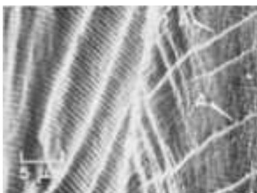
Fig. 880 High-magnification view of the fatigue precrack produced in air at base of notch in specimen in Fig.
