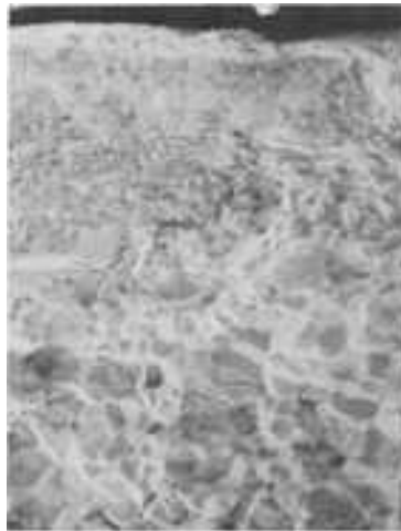
Fig. 540 Brittle intergranular fracture of AISI 9254 due to quench cracking. The crack initiated at a seam, 0.15 mm (0.006 in.) deep. The seam wall is the irregularly textured area at top in the fractograph. SEM, 200× (J.H. Maker, Associated Spring, Barnes Group Inc.)
