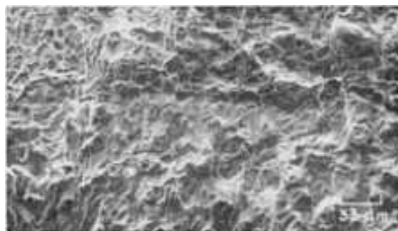
Fig. 807 SEM view, at higher magnification, of the fracture surface shown in Fig. 806, with the fatigue-crack surface at bottom and the fast-fracture surface at top. Note the secondary cracks and lack of clear fatigue striations in the fatigue area. See also Fig. 808. 300×
