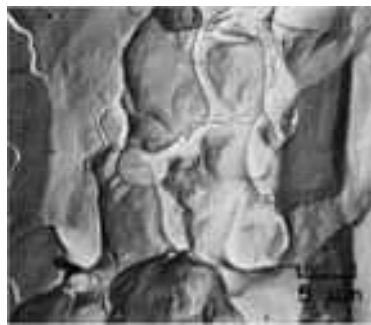
Fig. 1177 Surface of a fracture in a specimen of titanium alloy Ti-7Al-1Mo-1V that was broken in a drop-weight tear test, consisting mostly of dimples. A feature that apparently is a tear ridge (vertical) is visible at far right. TEM p-c replica, 2000×
