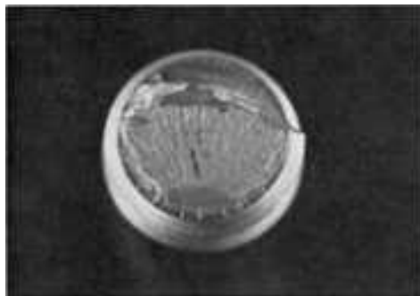
Fig. 726 Low-cycle fatigue fracture in threaded specimen of 13-8 PH stainless steel (tensile strength): 1634 MPa, or 237 ksi; 47% reduction of area) tested in tension-tension ( R = 0.1 ) with maximum loading at 60% of tensile strength. Fracture, at 16,000 cycles, began at lower edge of crescent-shaped area at bottom. 6×
