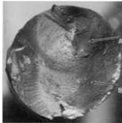
Fig. 394 Torsion-overload fracture in AISI 4340 steel oil quenched from 845 °C (1550 °F) and tempered at 635 °C (1175 °F) to a tensile strength of 931 MPa (135 ksi). In general, the fracture surface is flat and shiny. See Fig. 395 and 396 for TEM views of areas A and B.
