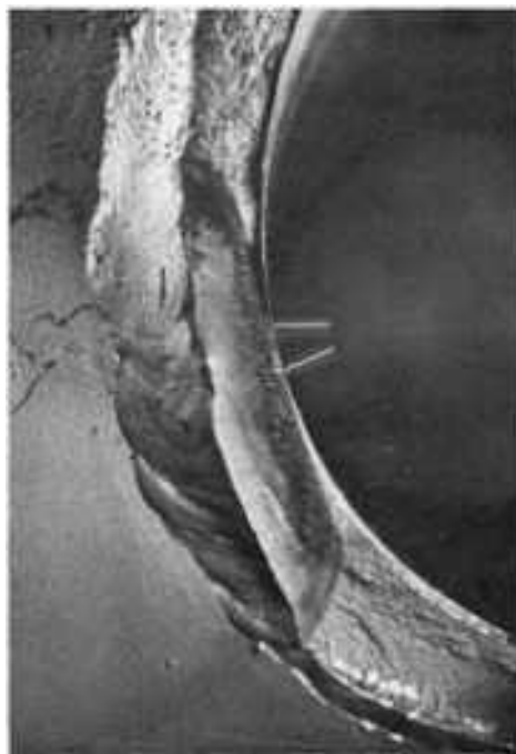
Fig. 450 Fracture surface of the barrel portion of the broken hub in Fig. 449, showing the fatigue-crack origin. The fatigue crack was about 44 mm ( 1\frac{3}{4} in.) long, but had penetrated the hub wall completely for only about 3.2 mm ( \frac{1}{8} in.) (arrows). Note shear lip at inside of hub wall on either side of the fatigue crack. 2×
