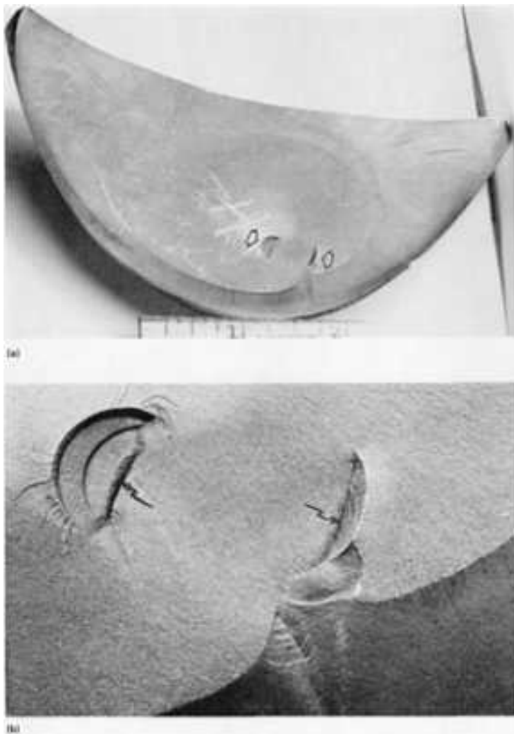
Fig. 56 Circular spall from the shoulder of a forged, hardened alloy steel mill roll with two small fatigue origins. A subsurface crack connected the two fatigue zones. Note that the spall surface is relatively featureless. (a) About
