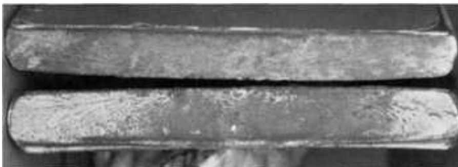
Fig. 500 Mating fracture surfaces of the broken main-landing-gear spring leg in Fig. 499. A small fatigue zone
