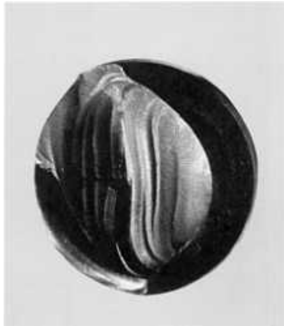
Fig. 769 Surface of a low-cycle fatigue fracture in the collar of a rivet-heading tool of AISI S1 tool steel heat treated to a hardness of 56 to 58 HRC. Following the development of the smooth fatigue zone at right, fracture occurred in a few hours of service, generating the unusual beach marks at center and left. 2×
