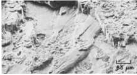
Fig. 1055 An area of the corrosion-fatigue fracture surface of an aluminum alloy 7075-T651 that was tested in a 3.5% NaCl solution under a cyclic stress-intensity range ( \Delta K ) of 6.6 \text{ MPa}\sqrt{m} ( 6 \text{ ksi}\sqrt{in} ) at 10 cps. Ductile and brittle striations would be expected in such a fracture, but cannot be resolved at this magnification. See also Fig. 1056. SEM, 120×
