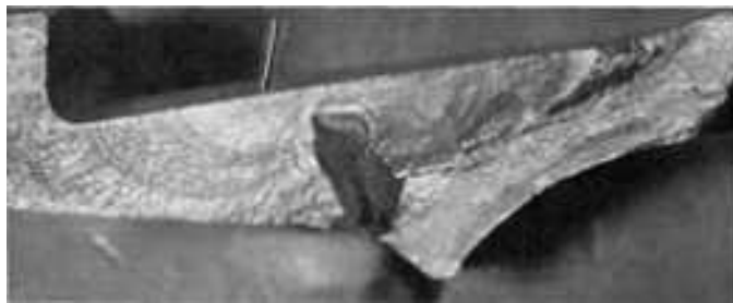
Fig. 969 View of an area of one fracture surface of the broken hub in Fig. 968, showing the fatigue-crack origin. Visible are beach marks, which suggest that the origin is at the location marked by the arrow, presumably at one of several corrosion pits that were found on the surface of the hub. After having penetrated a short distance, the fatigue crack developed a step (dark facet); a second fatigue crack originated at one end of the step. 1.8×
