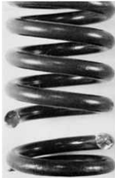
Fig. 262 Fatigue-fractured valve spring of 4.8-mm ( \frac{3}{16} -in.) diam AISI 1060 steel wire. The wire appears to be free of surface defects, a conclusion that is supported by the evidence in Fig. 263. 2×
