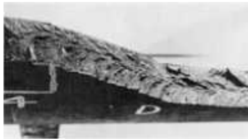
Fig. 183 View of the bottom segment of the fractured shell in Fig. 177, showing an area opposite the one in Fig. 182. This view also reveals sharply defined chevron marks that point to the right. 0.45×
