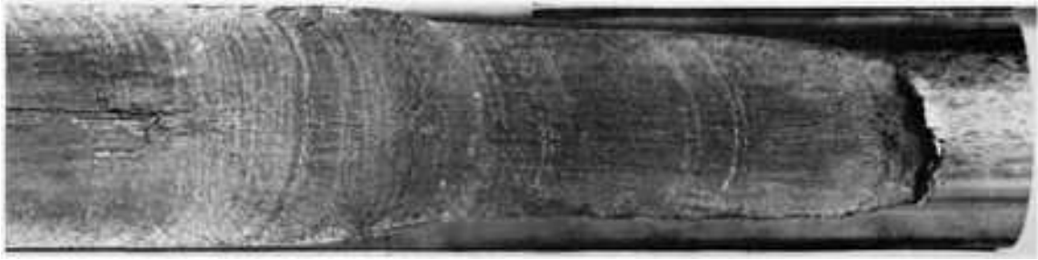
Fig. 205 Fatigue-fracture surface of the shaft of a forging hammer of AISI 1144 steel containing 0.45% C, 1.60% Mn, and 0.28% S. The fatigue crack began at a heavily abraded surface area (out of view to the left), penetrated to the center of the shaft, then turned 90° and propagated longitudinally to the point of termination at right (about 635 mm, or 25 in.). See also Fig. 206. ~0.5×
