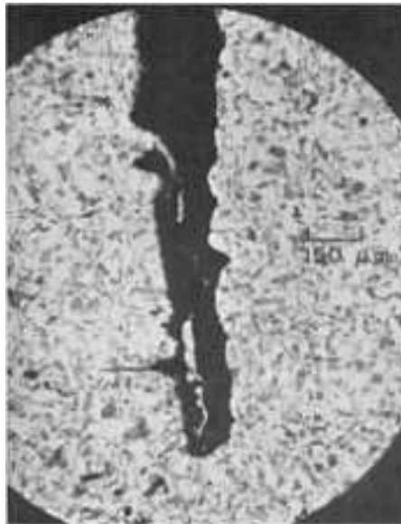
Fig. 156 Section of the fractured shaft shown in Fig. 151, revealing the bottom of one of the corrosion-fatigue cracks. Note that corrosion blunted the tip of the main crack but not the tip of the sharp secondary crack at left, which formed later. Picral etch, 67×
