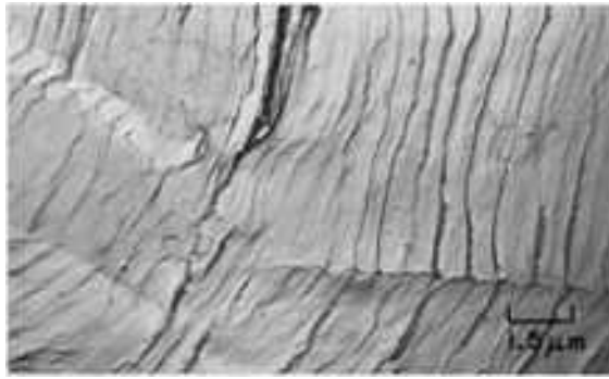
Fig. 625 TEM p-c replica of another area near C in Fig. 618, showing a further increase in fatigue-striation spacing. A junction of two crack fronts is visible at lower right. Secondary cracks appear to have formed at some striations. 6500×
