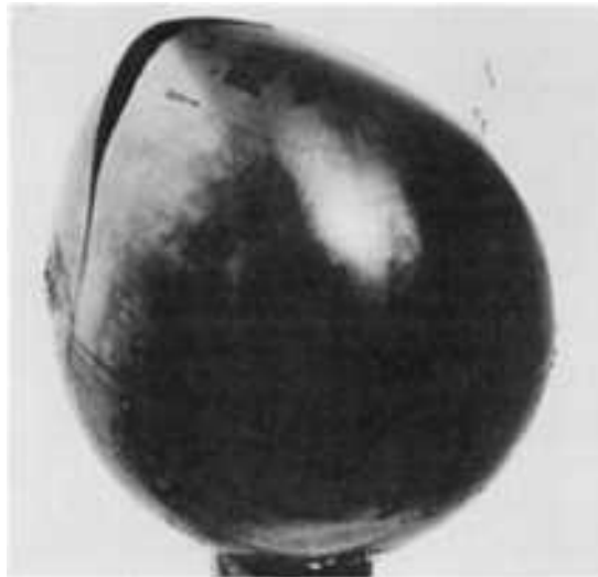
Fig. 19 Macrograph showing ductile overload fracture of a high-pressure steel vessel tested at room temperature. See also Fig. 20.
