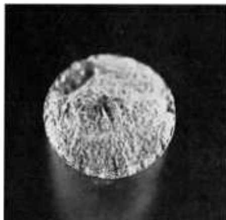
Fig. 1021 Cone-shaped fracture surface produced by low-cycle fatigue in aluminum alloy 7075-T6 (same mechanical properties as in Fig. 1015). Loading was tension-tension with R = 0.1 and a maximum loading of
