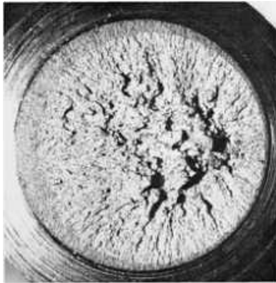
Fig. 431 Tension-overload fracture in a notched specimen same as in Fig. 429 and 430, but tested at -155^{\circ}\text{C} ( -245^{\circ}\text{F} ). Even at this very low temperature, a small annular zone of fibrous fracture was formed next to the notch. Final fast fracture produced the radial marks in the central region. 17\times
