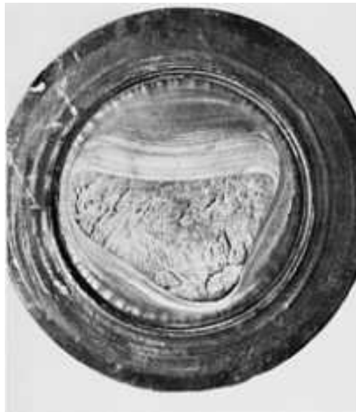
Fig. 521 Surface of a fatigue fracture in a 200-mm (4-in.) diam axle of AISI 8640 steel with a hardness of approximately 30 HRC. Contained within a shrink-fitted collar (visible here), the nonrotating axle was subjected to bending stresses in three directions, which produced this unusual pattern of beach marks. 0.65×
