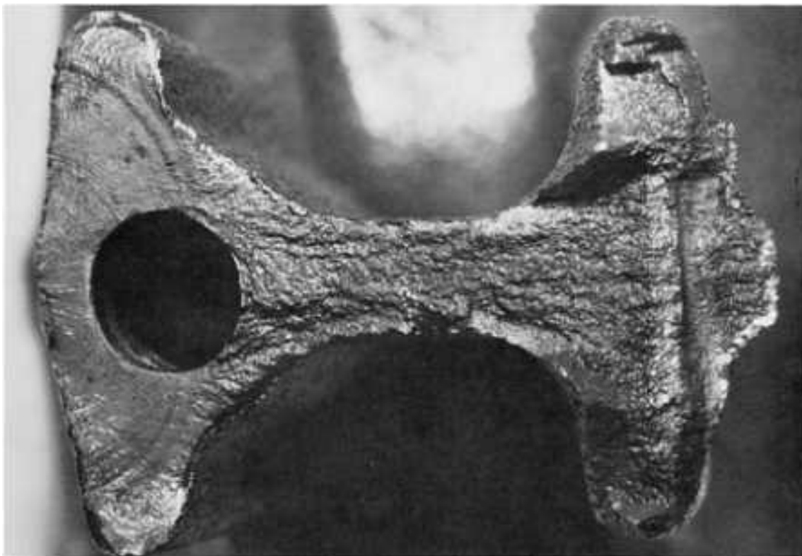
Fig. 523 Surface of a fatigue fracture in a forged connecting rod of AISI 8640 steel with a hardness of 26 to 27 HRC throughout. The rod broke after approximately 84,000 km (52,000 miles) of service. The fatigue-crack origin is at the left edge, at the flash line of the forging, but no unusual roughness of the flash trim there was discovered. No metallurgical cause of the fracture was detected. The fatigue crack progressed about halfway around the oil hole at left before final fast fracture occurred. Note the pronounced shear lip at the right edge. \sim 7\times
