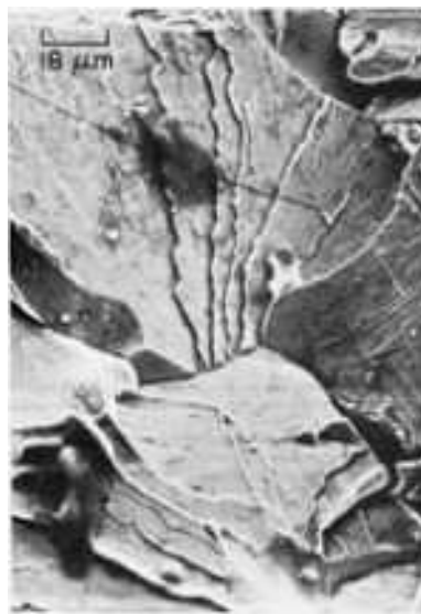
Fig. 1203 Surface of a slow-bending fracture that was produced at -130 °C (-200 °F) in an Fe-0.3Ni alloy that had been melted, deoxidized, forged, rolled, and heat treated exactly the same as the higher-nickel alloy shown in Fig. 1201 and 1202. See also Fig. 1204, 1205, and 1206. SEM, 550 \times
