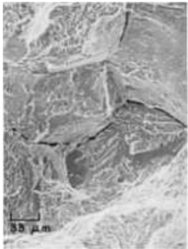
Fig. 560 Another area of the fracture surface, shown at higher magnification. This area has many characteristics of an intergranular fracture. Grain surfaces exhibit fine dimples, but no river patterns. SEM, 300×
