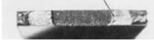
Fig. 1247 Surface of a high-cycle fatigue fracture in a stress-relieved specimen of 90Ta-10W alloy sheet containing a central transverse notch 5 mm (0.2 in.) wide. Tensile strength was 552 MPa (80 ksi). The specimen was loaded in tension at room temperature to a stress cycled from 80 to 400 MPa (11.6 to 58 ksi) at 1000 cycles/min and broke after 15,900 cycles. Considerable necking accompanied fast fracture. See also Fig. 1248 and 1249 for TEM replicas of areas at the arrow. 6×
