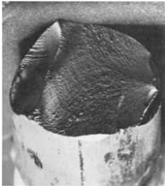
Fig. 772 An impact fracture in a 44-mm ( 1 \frac{3}{4} in.) diam notched bar of AISI T1 tool steel that was broken for inspection same as the bar in Fig. 771. The crack resulting from the first hammer blow, which started at the notch at right, shows the network of intersecting fine markings called "Wallner lines." The crack that resulted from the second hammer blow is at left. 1.9×
