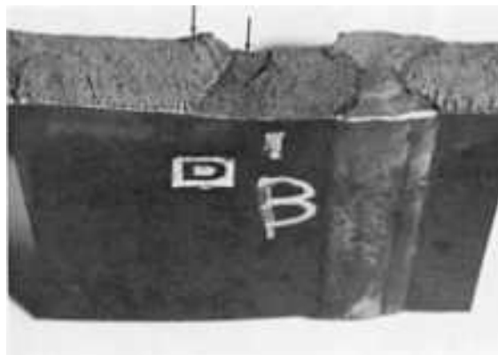
Fig. 173 Same portion of the shell plate as in Fig. 172, but before sectioning and at a different orientation. The two dark crescents partly visible at top edge of the fracture surface (at arrows) were caused by arc strikes and served as crack nuclei. 0.7×
