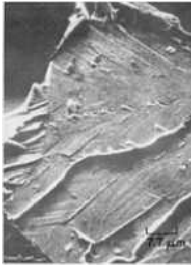
Fig. 1206 Another view of the bending fracture in Fig. 1205, showing a different region at higher magnification. This region best demonstrates the difference between this Fe-0.3Ni alloy and the Fe-3.9Ni alloy in Fig. 1201 and 1202 by displaying many small "tongues," or microtwins, which are characteristic of Fe-0.3Ni and also of unalloyed (Armco) iron, but not of Fe-3.9Ni. SEM, 1300×
