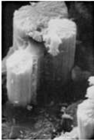
Fig. 1309 Fracture surface of a carbon/epoxy "wet" specimen tested at 25 °C (77 °F) at a moisture contents of 2.0 wt%. Fractograph shows typical appearance of a local failure of two fibers where the fracture originated at the point of contact between the two fibers. SEM (same conditions as in Fig. 1294), 2000× (The composite specimens shown in Fig. 1296, 1297, 1298, 1299, 1300, 1301, 1302, 1303, 1304, 1305, 1306, 1307, 1308, 1309, and 1310 all consisted of circa 1978 Thornel 300 fibers in Narmco 5208 epoxy resin. The composites were all fabricated by lay-up of prepreg tape and were autoclave cured 175 °C (350 °F) according to the manufacturer's recommendations. Specimens were then end-tabbed and cut in accordance with the ASTM D3039. The 0° and 90° tensile specimens were tested in accordance with ASTM D3039, and the 0° flexural three-point-bend specimens were tested in accordance with ASTM D790. The composites were dried before testing in the same manner as the epoxy specimens described in Fig. 1294 and 1295. "Dry" specimens were tested as-dried and had essentially 0 wt% moisture. "Room" moisture specimens had about 0.6 wt% moisture, having been placed after drying in a chamber at 60 °C (140 °F) and 60% relative humidity for at least 2 months and then placed in a drawer in the laboratory for several months before testing. "Wet" specimens had about 1.5 to 2.0 wt% moisture, having been placed for several months in an environmental chamber at 60 °C (140 °F) and 100% relative humidity. The composites were tested at moisture conditions designed not to alter their conditioning, and at the temperatures noted.) (L. Clements, San Jose State University, and P.R. Lee, United Technologies)
