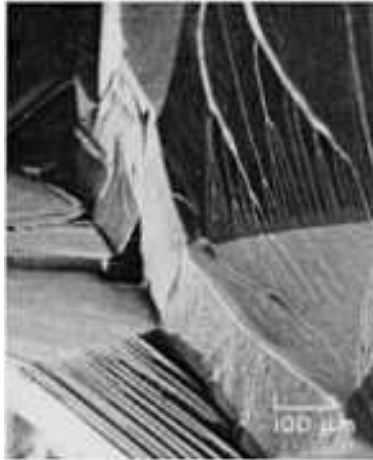
Fig. 1223 Room-temperature tensile fracture by cleavage of an Fe-6.2Ta alloy solution treated 1 h at 1400 °C (2550 °F), water quenched, aged 1 h at 700 °C (1290 °F) and air cooled. Laves-phase \text{Fe}_2\text{Ta} precipitate, uniformly distributed in the matrix and believed present at grain boundaries, caused brittleness (<1% tensile elongation). See also Fig. 1224. SEM, 100×
