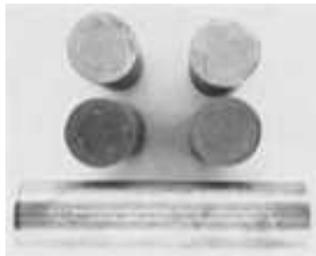
Fig. 114 Example of specimens used in the Shepherd P-F test. The 19-mm ( \frac{3}{4} -in.) diam, 100-mm (4-in.) long specimen is shown at the bottom. The test consists of fracturing an austenitized and brine-quenched specimen. Case depth can be observed on the fracture. After fracture grain size is rated, the fracture surface is carefully ground off. Macroetching then reveals the depth of hardening. Superficial hardness tests are used to determine the case depth to a particular hardness.
