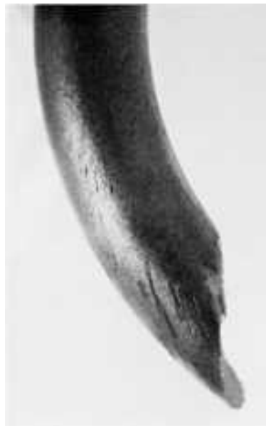
Fig. 265 Fractured 13-mm ( \frac{1}{2} -in.) diam spring of AISI 10B62 steel wire with a hardness of 477 HB. Note the spiral gouges, which are screw marks that were generated during coiling. See also Fig. 266. 2×
