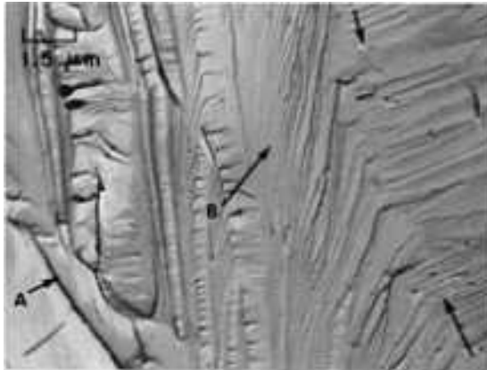
Fig. 1245 TEM p-c replica of an area at the arrow in Fig. 1244. Here, the fracture surface shows transgranular cleavage. Tilt boundary at A; elsewhere, twist boundaries (between arrows) and suggestions of cleavage feather marks (at B). 6500×
