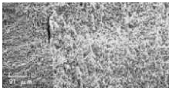
Fig. 1154 Fracture surface of a fracture-toughness specimen of titanium alloy Ti-6Al-4V heat treated 40 min at 955 °C (1750 °F) and water quenched, aged at 510 °C (950 °F), and tested in hydrogen. (Structure is continuous \beta phase with dispersed \alpha phase.) The fatigue-precrack region is at left. The tensile-overload region, at right, closely resembles that of the specimen in Fig. 1158. SEM, 110×
