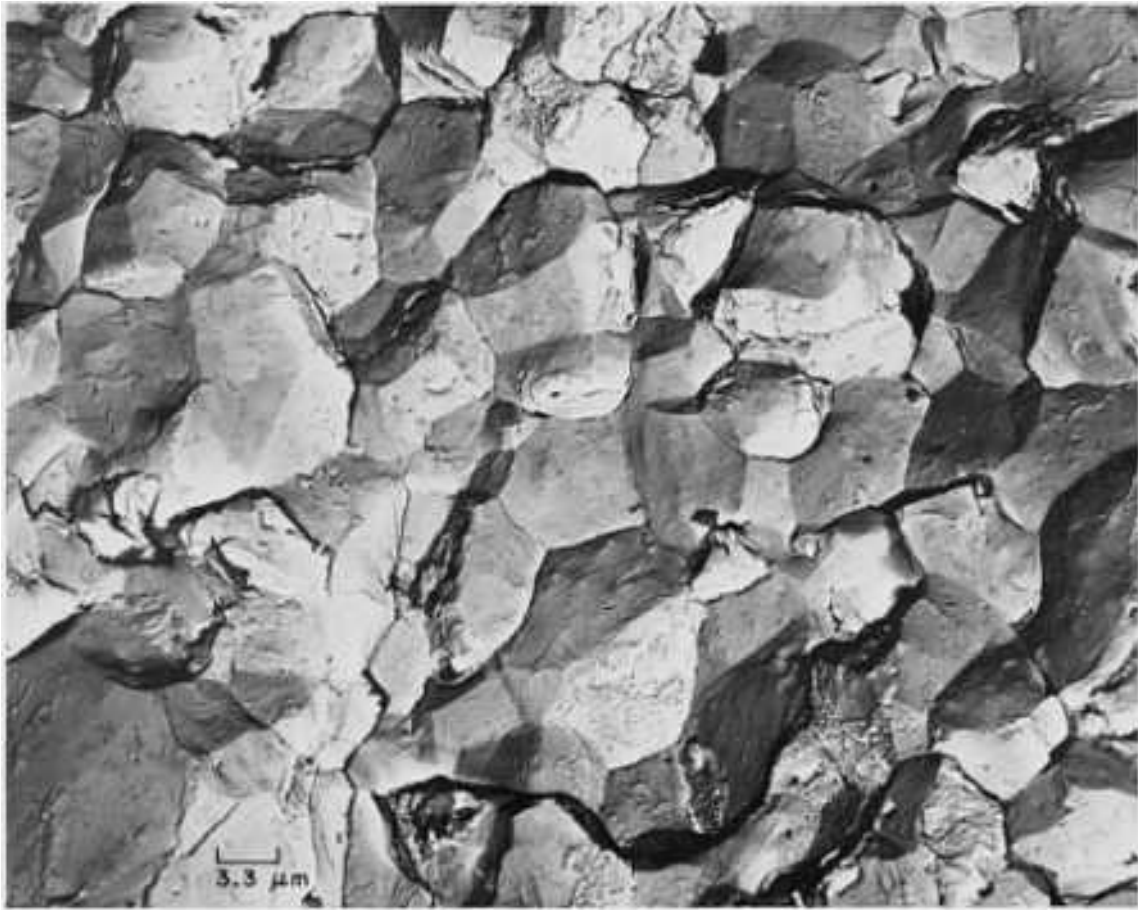
Fig. 470 Higher-magnification view of fracture surface at arrow in Fig. 469, showing clearly the intergranular nature of the fracture, which resulted from stress-corrosion cracking. Grains generally are equiaxed, and the fracture has closely followed grain boundaries. TEM p-c replica, 3000×
