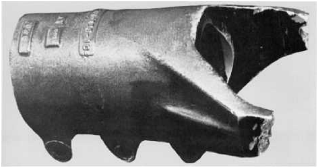
Fig. 929 A broken extension-housing yoke, part of a helicopter tail-rotor drive assembly, that fractured by fatigue in service. The fracture occurred through the left and right lugs at the points of attachment to the tail boom. The yoke was cast from aluminum alloy 356.0 and heat treated to the T6 temper. Chemical analysis showed that the composition of the yoke conformed to specifications, except for silicon, which was 0.05% below the required minimum. Hardness measurements ranged from 48 to 52 HRB (or about 81 to 85 HB), which was above the required minimum. Details of the fractures are shown in Fig. 930, 931, 932, 933, 934, 935, 936, 937, and 938. Actual size
