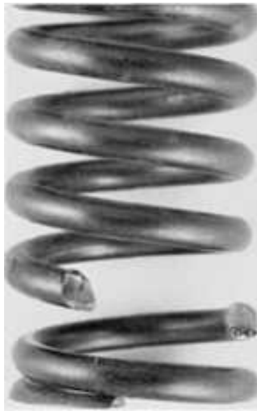
Fig. 269 Fatigue-fractured spring of 5-mm (0.200-in.) diam AISI 1060 steel wire (hardness, 43 to 48 HRC). This fracture, unlike that of the similar spring in Fig. 261, originated at the surface (see Fig. 270). 1.7×
