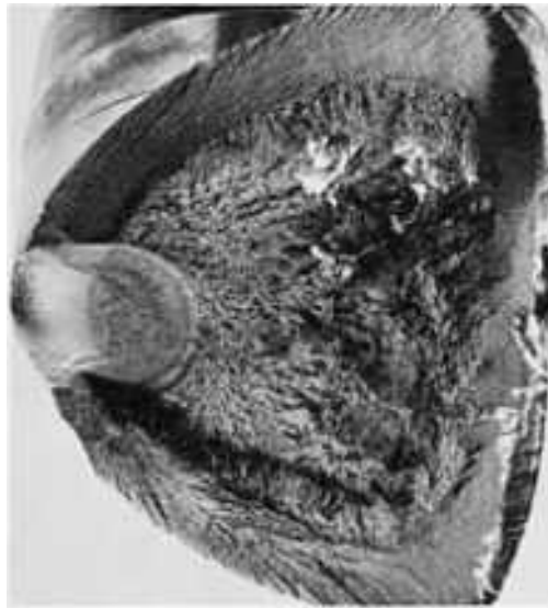
Fig. 195 Surface of a fatigue fracture in an induction-hardened axle of AISI 1041 steel with a hardness of 46 HRC in the hardened zone. The fatigue crack originated at a fillet (with a radius smaller than specified) at a change in shaft diameter near a keyway runout. Note the two sets of chevron marks along the hardened perimeter, each set pointing to the crack origin at left. Actual size
