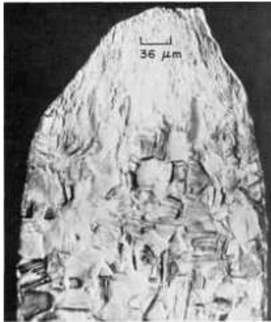
Fig. 919 Longitudinal section through a tension fracture in a warp wire of a Fourdrinier wire cloth of phosphor bronze C. Slip lines are visible throughout the microstructure. Plastic flow and reduction in area at the fracture (top) were attributed to excessive warp tension, \text{FeCl}_3 etch, 265×
