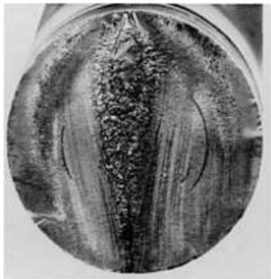
Fig. 217 Reversed bending fatigue of a 40-mm (1.6-in.) diam AISI 1046 steel shaft (30 HRC). Note the symmetrical fatigue pattern of beachmarks on each side, with the final rupture on the diameter. This indicates that each side of the shaft was subjected to the same maximum stress and to the same number of load applications. (D.J. Wulpi, Consultant)
