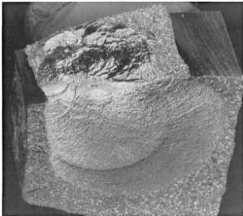
Fig. 308 Deep "shell crack" and "detail fracture" in head of railroad rail removed from service. Composition of standard carbon rail steel: 0.60 to 0.82% C, 0.70 to 1.00% Mn, and 0.10 to 0.23% Si. Gage side of rail is at left. A 5- to 10-mm ( \frac{1}{4} - to \frac{3}{8} -in.) thick layer has been removed from the running surface to expose the shell crack (top). Deep shells such as this one typically nucleate at stringers or microinclusions and propagate approximately parallel to the running surface. Some shells form a branch crack, or detail fracture, in the transverse plane (lower portion of figure) that can cause a service break if not detected in time. Detail fractures typically have featureless crack propagation surfaces, but may exhibit beach marks (as in this example) that reflect the traffic pattern or temperature (thermal stress) changes during service. See also Fig. 309 and 310.
