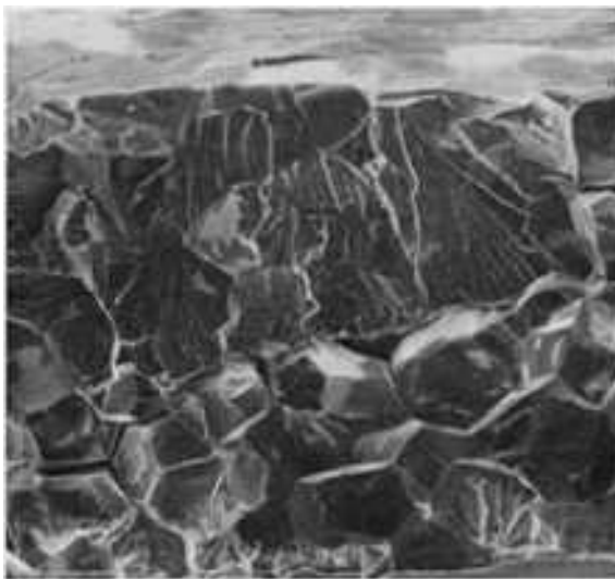
Fig. 1090 The external surface (top) and the corrosion-fatigue fracture surface (bottom) of a solution-treated and peak-aged Al-5.6Zn-1.9Mg sample tested in deaerated 0.5 mol NaCl at a cathodic potential of -1.6 V (SCE). Compare with Fig. 1089, 1093, and 1095. SEM, 100× (R.E. Ricker, University of Notre Dame, and D.J. Duquette, Rensselaer Polytechnic Institute)
