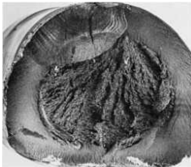
Fig. 196 Surface of a bending-plus-torsional-fatigue fracture in an experimental 89-mm ( 3\frac{1}{2} -in.) diam tractor axle of AISI 1041 steel that had been induction hardened. Fracture occurred after 1212 h on an endurance-test track. Note beach marks fanning out from the fatigue-crack origin (slightly to left of center, at top). Beyond the beach marks, cracking progressed by fast fracture along the hardened perimeter, producing two sets of chevron marks pointing toward the crack origin (like the chevron marks in Fig. 195). See also Fig. 197. 1.25×
