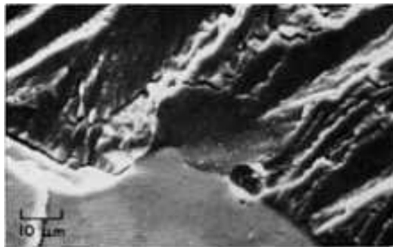
Fig. 1059 The area outlined by the rectangle in Fig. 1058, as seen at ten times the magnification there, which makes the fine fatigue striations in the smooth region clearly visible. Above are brittle striations forming, at a steep incline, what is in effect a cleavage step up to a second fracture level. SEM, 1000×
