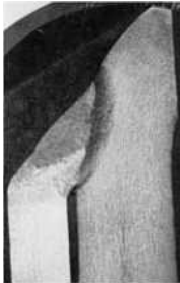
Fig. 17 A properly illuminated section through a weld. Vertical lighting was used to reveal flow lines in the base metal, the heat-affected zone, and the successive weld beads. Base metal was 1018 steel, component, an axle housing. Photomicrograph. Etched in ammonium persulfate. 4×
