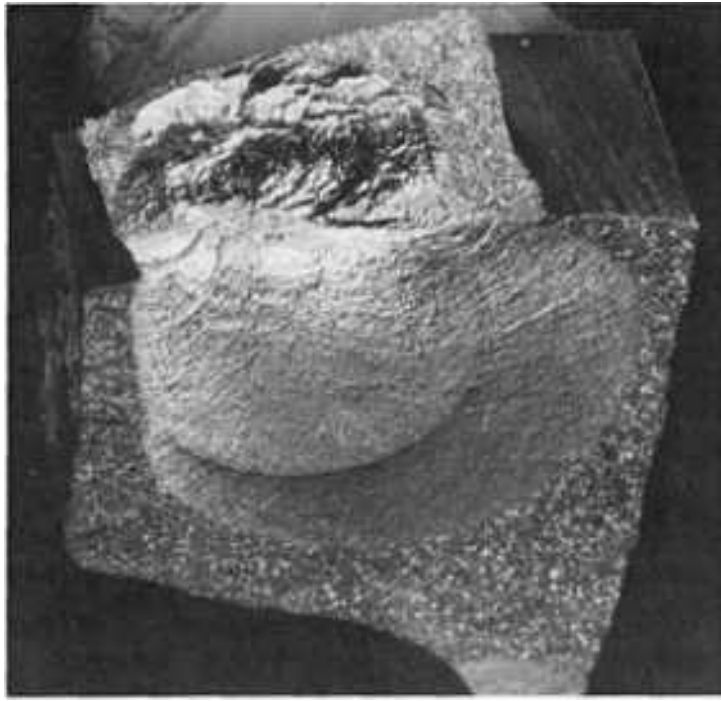
Fig. 69 Macrograph of broken rail showing the interconnection between the shell fracture (across the top) and the detail fracture (on the transverse plane). 3.5×. (R. Rungta, Battelle Columbus Laboratories)
