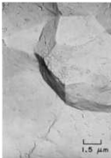
Fig. 399 TEM p-c replica from a different region in area A (the quench-crack crescent) in the fracture surface shown in Fig. 397. Here, as well as in Fig. 398, the crack path has been along the grain interfaces. Scattered marks here resemble the hairline indications associated with either hydrogen embrittlement or stress-corrosion cracking. 6500×
