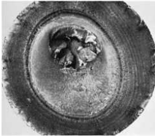
Fig. 193 Surface of a fatigue fracture in a shaft of AISI 1040 steel with a hardness of approximately 30 HRC. The shaft was fractured when subjected to rotating bending. The oval shape of the central region of final fast fracture indicates that two mutually perpendicular, unequal bending stresses were present. The ratchet marks around the perimeter of the shaft indicate that fracture began at several points. 1.63×
