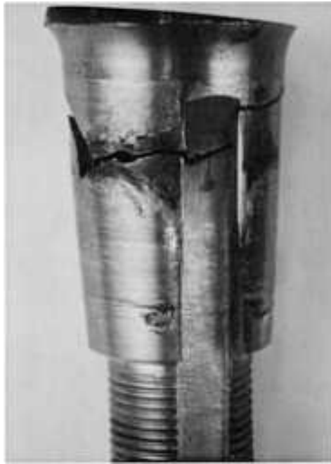
Fig. 203 View of a broken keyed spindle of AISI 1041 steel with a hardness of 333 HB. A large amount of fretting is visible on both sides of the fracture. Note that the radius of the keyway edge seems small near the fracture. See also Fig. 204. 1.5×
