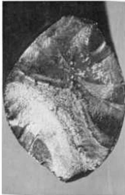
Fig. 341 Surface of a fatigue fracture in a suspension component of AISI 4140 steel heat treated to a hardness of 273 HB. Two fatigue zones are evident, at lower left and at upper right; the remainder of the fracture surface is the zone of final fast fracture. 5×
