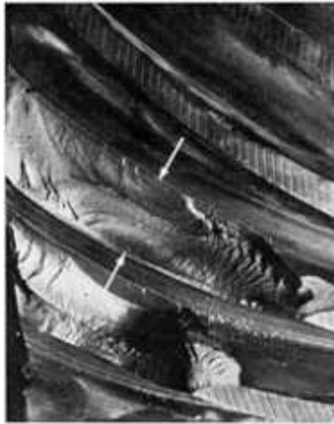
Fig. 477 Fatigue fractures in a spiral bevel pinion gear of AISI 4820H steel, case hardened to a depth of 1.1 to 2.0 mm (0.045 to 0.080 in.). Case hardness, 56 HRC; core hardness, 30 HRC. Fatigue cracks began in tooth roots (which were not shot peened), often forming on either side of a tooth (arrows) and meeting in the middle of the tooth. A deeper case and shot peening of the entire gear were recommended. Actual size.
