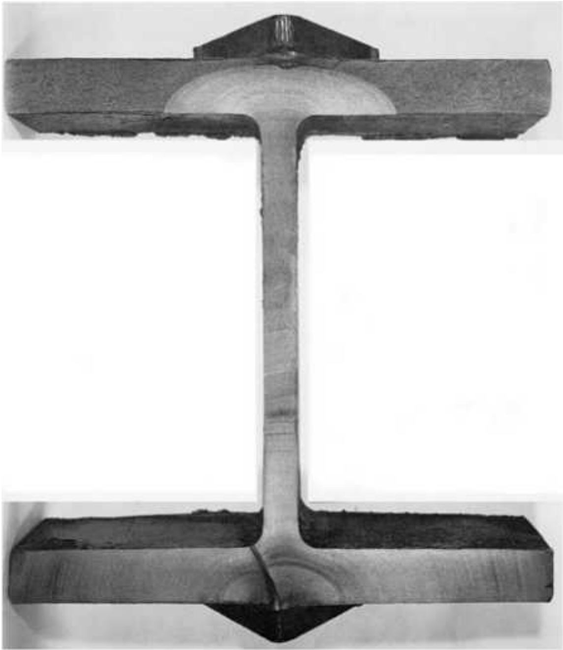
Fig. 208 Another view of the fatigue-fracture surface of the medium-carbon steel I-beam in Fig. 207. The fracture origins are clearly evident in the flange at bottom, where two nuclei are situated at the toe of the weld joining a reinforcement plate to the flange. It is remarkable that the fatigue crack penetrated the entire flange at bottom, the entire web, and part of the flange at top before final fast fracture occurred. See also Fig. 209 and 210. 0.5×
