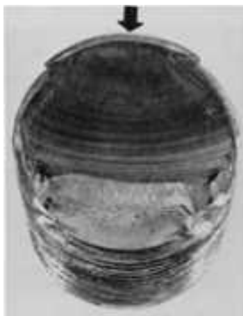
Fig. 50 Fatigue failure of a bolt due to unidirectional cycling bending loads. The failure started at the thread root (arrow) and progressed across most of the cross section before final fast fracture. Actual size.
