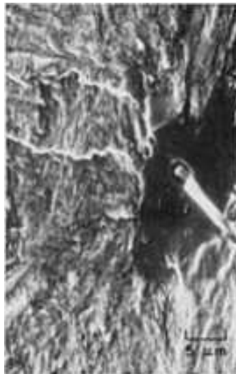
Fig. 387 Higher-magnification view of the inclusion (fracture origin) shown at center in Fig. 386. Little evidence of fatigue striations is found this close to the origin. See also Fig. 388. SEM, 2000×
