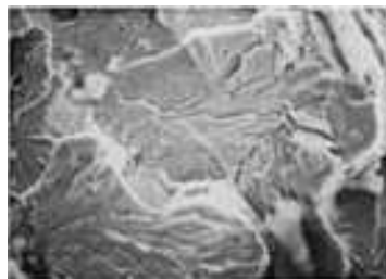
Fig. 12 Cleavage in a low-carbon steel specimen that was impact fractured at liquid-nitrogen temperatures. 385×
