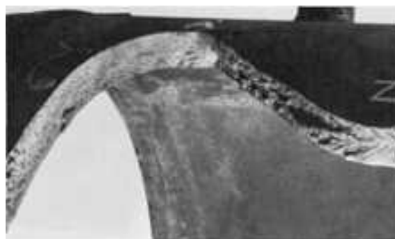
Fig. 181 View of the far left end of the top segment of the fractured pressure-vessel shell in Fig. 177, showing chevron marks. The chevron marks were smeared subsequent to fracture, but can be clearly identified as
