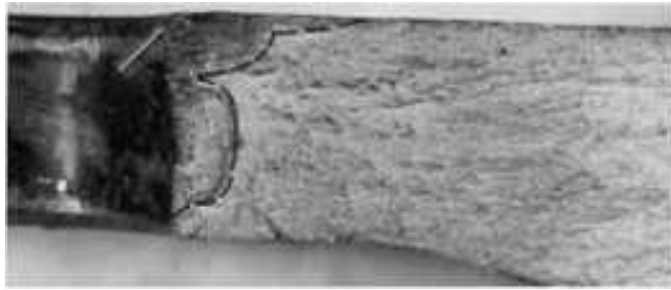
Fig. 1082 Fracture surface inboard of the bolthole in the clevis-attachment lug in Fig. 1081. The primary stress-corrosion crack, which originated at the arrow, and which is enclosed by the dashed line, is larger than that in Fig. 1080. This actuator beam had hardness normal for 7079-T6: 152-157 HV (10-kg load). 4×
