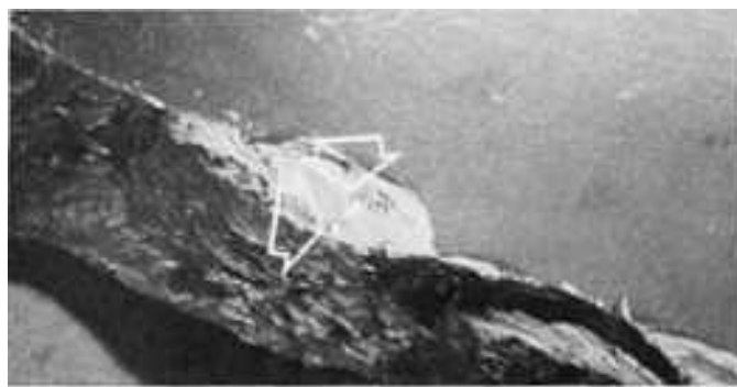
Fig. 973 Fracture surface of the broken hub in Fig. 970, showing an area of the circumferential separation between the hub and web. Bright flakes, similar to the defect that initiated the fatigue crack in Fig. 972, are visible at the arrows. These defects have been attributed to hydrogen damage. Actual size
