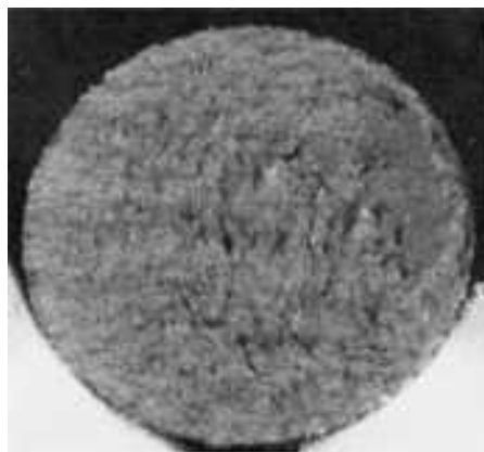
Fig. 1018 Tension-overload fracture in notched specimen of aluminum alloy 7075-T6. Notched tensile strength, 750 MPa (109 ksi); unnotched tensile strength, same as in Fig. 1015. Surface is flat and coarsely fibrous. Considerable secondary cracking is evident, even at this low magnification. See also Fig. 1019 and 1020. 9×
