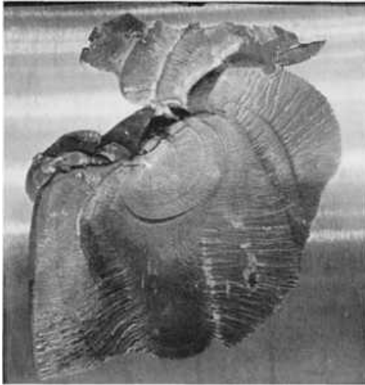
Fig. 57 Circular spall on the surface of a forged, hardened alloy steel mill roll. The arrow indicates the fracture origin. Note the fatigue marks showing the growth away from the origin, followed by brittle fracture. 0.68×
