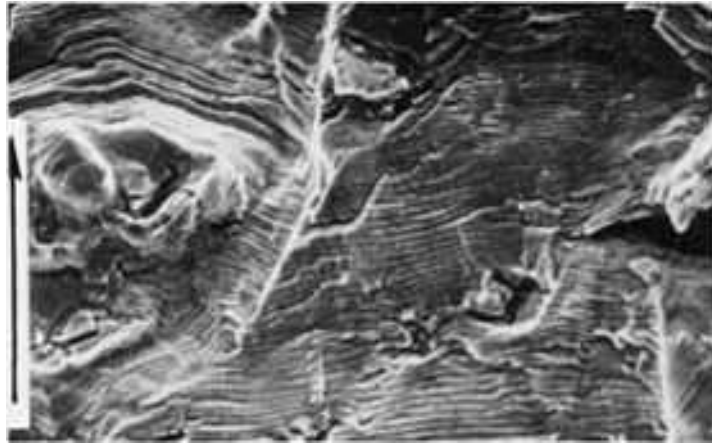
Fig. 92 Fatigue fracture appearance of Inconel X-750 tested in air at 650 °C (1200 °F) at \Delta K = 35 \text{ MPa}\sqrt{m} (32 ksi \sqrt{in} ). The fracture path is transgranular with ductile fatigue striations. The crack propagation direction is indicated by arrow. Compare with the fracture appearance of the same alloy shown in Fig. 90(a), which was tested at \Delta K = 20 \text{ MPa}\sqrt{m} (18 ksi \sqrt{in} ). Source: Ref 245
