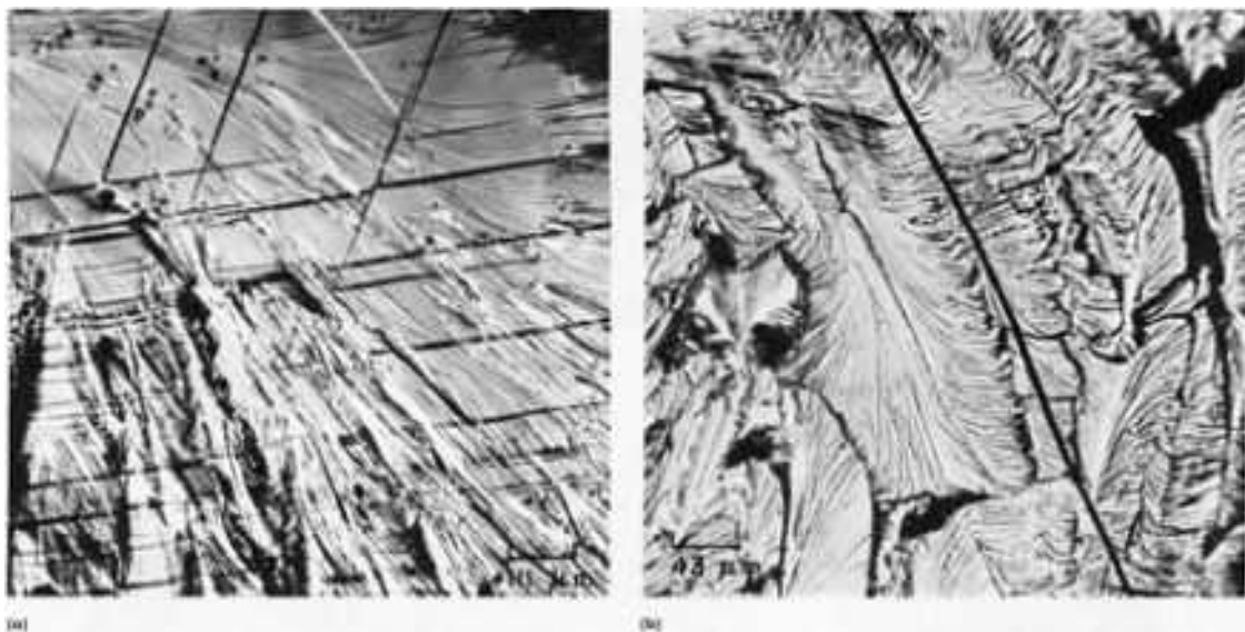
Fig. 5 Cleavage fractures in room-temperature impact specimens examined by C.A. Zapffe. (a) Cast polycrystalline antimony (99.83Sb-0.04S-0.035As-0.035Pb-0.015Fe-0.01Cu) (b) Vacuum-arc-cast high oxygen
