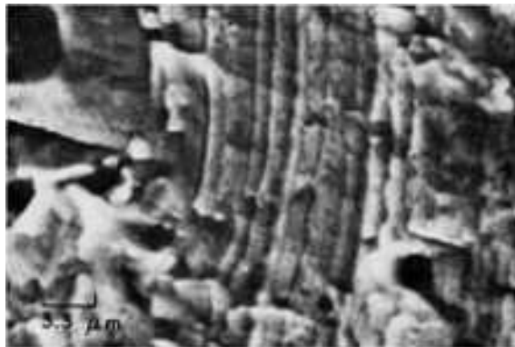
Fig. 1030 Highly magnified view of fatigue striations typical of those in areas A in Fig. 1027. In general, these striations were parallel with the flaw B-B. Dimples characterized the remainder of the fracture. Inclusions near the flaw suggested that it was the result of a pipe not cropped from the ingot. SEM, 3000×
