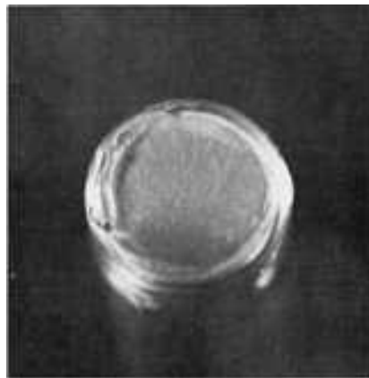
Fig. 1171 Highly-cycle fatigue fracture in a specimen of titanium alloy Ti-6Al-4V (same mechanical properties as in Fig. 1162) that was tested in tension-tension ( R = 0.1 ) at maximum loading of 345 MPa (50 ksi), breaking in 937,000 cycles. The curved fatigue beach mark can be seen near bottom. See also Fig. 1172 and 1173. 6×
