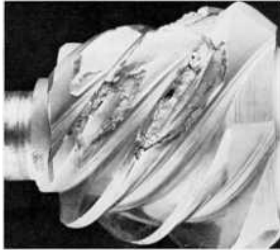
Fig. 475 Companion gear to that in Fig. 474 (carburized AISI 4817 steel) showing subcase fatigue fractures initiated by fine cracks similar to those in Fig. 474. Large fragments have spalled away from the teeth. Fatigue beach marks can be seen in these complex fracture surfaces, especially at upper right. Actual size.
