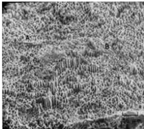
Fig. 1251 Higher-magnification view of the area in the larger rectangle in Fig. 1250. At A are two transversely oriented features that appear to be graphite fibers that either are lying loose on the surface or were inadvertently misaligned during manufacture. The feature at B is probably a ridge. Much of the surface exhibits broken fibers, the ends of which are roughly in the same plane as the fracture in the surrounding matrix, but at center are exposed fibers with the appearance of "palisades." SEM, 180×
