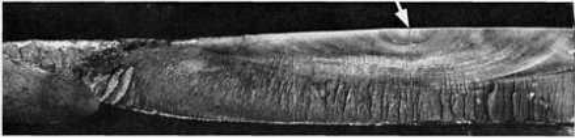
Fig. 245 Surface of a fatigue fracture that occurred, after 732 h of service, in a tooth of the induction-hardened AISI 1053 steel left-side bull gear of a tractor. Hardness of the tooth was 57 HRC at the tip and 50 HRC at a depth of 13.3 mm (0.52 in.). Hardness in the root fillet was approximately 56 HRC near the surface and 50 HRC at a depth of 11.5 mm (0.45 in.). The arrow indicates the origin of the fatigue crack. See also Fig. 246, 247, and 248. ~2.5×
