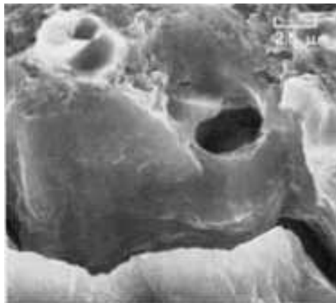
Fig. 1020 Higher-magnification view of the area in the rectangle in Fig. 1019. This fourfold enlargement makes visible the fine dimples surrounding the particle sites. Note that the surfaces of the secondary grain-boundary cracks are remarkably smooth. SEM, 4000×
