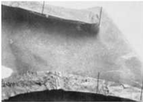
Fig. 840 Fracture surfaces of the two broken turbine-rotor blades at the bottom in Fig. 839. Fatigue beach marks are faintly visible at right on the fracture surface of the lower blade. The region between the parallel black lines on each blade was examined by electron microscopy. 6×
