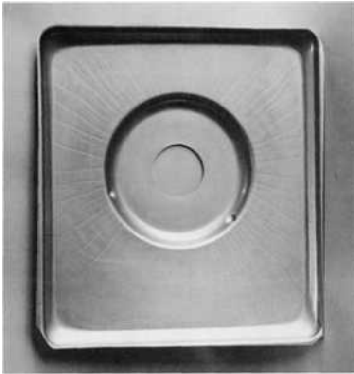
Fig. 90 Stretcher-strain marks (Lüders bands) on the surface of a range component after forming 0.25 ×.
