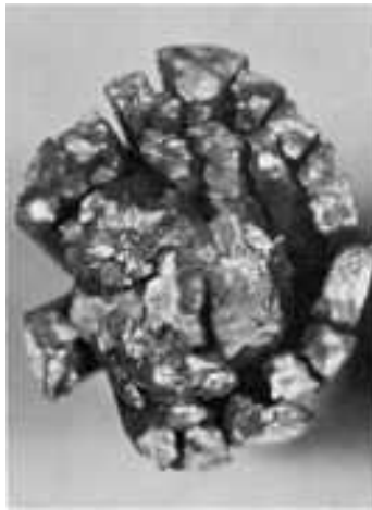
Fig. 527 Fracture surface of the left portion of the shaft in Fig. 525, showing the badly mangled splines separated by longitudinal cracks, which are evident also in Fig. 525. 1.25×
