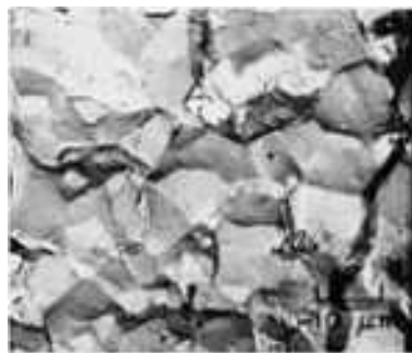
Fig. 417 TEM p-c replica of the fracture surface in Fig. 414, showing a region at the bottom of a depression directly below the surface crack. In this entire area of projections and depressions (see Fig. 414), fracture was completely intergranular. 1000×
