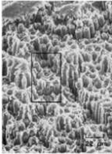
Fig. 1252 Higher-magnification view of the area in the smaller rectangle in Fig. 1250, showing "palisades," some of which are the reverse of those in Fig. 1251 in that the fibers have broken at the bottom of the "palisades," exposing the sides of the holes in the matrix. See Fig. 1253 for an enlarged view of the area in the rectangle. SEM, 450×
