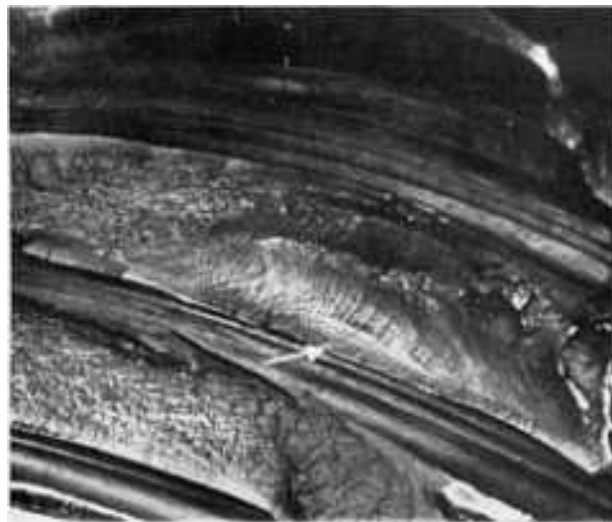
Fig. 514 Surface of a bending-fatigue fracture in a tooth (upper tooth in this view) of a large spiral bevel pinion of AISI 8620 steel carburized and hardened to 60 HRC at the surface. The arrow marks the fatigue-crack origin, in the root fillet. The absence of this tooth resulted in fracture of the tooth below by overload. 1.65×
