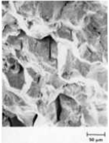
Fig. 94 Fracture appearance of a cold-worked type 316 stainless steel fatigue tested in vacuum of 593 °C (1100 °F) under a 1-min dwell time. Note the more intergranular nature of this fracture when compared to Fig. 89(b), which shows the fracture appearance of the same alloy tested under the same conditions, except at zero dwell time. Source: Ref 242
