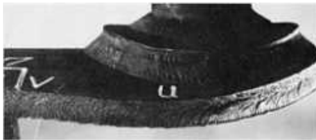
Fig. 184 View of the top segment of the fractured shell in Fig. 177, showing an area just to the left of the fracture origin. The continuity of the chevron marks that point toward location S (at right end) is much more perceptible here than in Fig. 179 because of a difference in illumination. 0.28×
