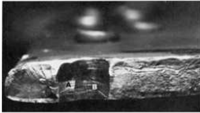
Fig. 976 Higher-magnification view of the rivet-hole area of the fracture surface shown in Fig. 975. The double-drilled nature of the rivet hole is shown quite clearly here. Two fatigue cracks originated at this hole--one beginning at arrow A and growing to the left, and the other beginning at arrow B and growing to the right. 5×
