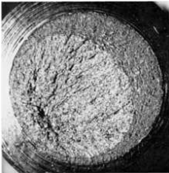
Fig. 430 Surface of a tension-overload fracture in a notched specimen of AISI 4340 steel the same as the specimen shown in Fig. 429, but tested at 80\text{ }^{\circ}\text{C} ( -110\text{ }^{\circ}\text{F} ). A fibrous zone, which originated at the notch, surrounds a radial zone, which is off-center because of nonsymmetrical crack propagation. 17\times
