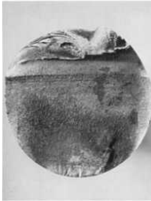
Fig. 340 Surface of a fatigue fracture in a stud of AISI 4140 steel with hardness of 34 HRC in the core and 45 HRC at the surface. The crack originated at the bottom in this view, in a well-rubbed fatigue zone, and penetrated nearly 90% of the cross section of the stud before final fast fracture occurred. 2×
