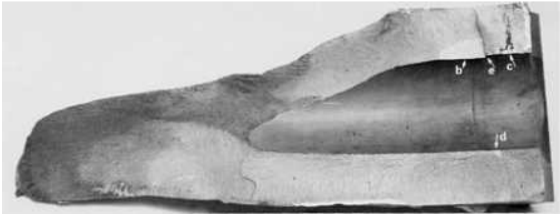
Fig. 1076 Surface of the fracture in the bogie beam shown in Fig. 1074. Three stress-corrosion cracks caused the final fast fracture, which was a tearing type of rupture. The intergranular attack characteristic of stress corrosion is shown in Fig. 1075. The three stress-corrosion cracks are the light areas marked by arrows "b," "c," and "d." The crack surfaces appear flat, but contain many small steps. Some of these steps were found to have been pulled away from the fracture surface in a leaf fashion, indicating overlapping or branching cracks. At arrow "e" is a pronounced step, which hides a portion of area "b." ~0.4×
