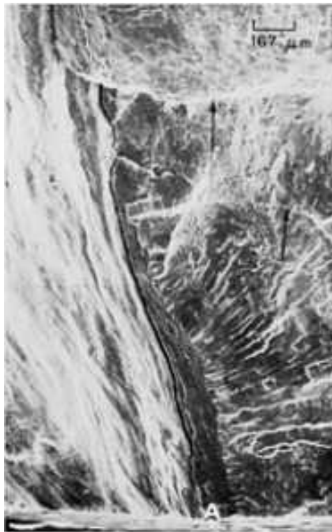
Fig. 1028 SEM view, at higher magnification, of the area at O in Fig. 1027. At left of the boundary (dark line running up from A) is the surface of the flaw (B-B in Fig. 1027); at right of it is a fatigue surface (A at right in
