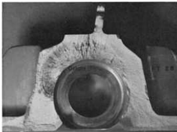
Fig. 14 Forged aluminum alloy 2014-T6 aircraft component that failed by fatigue. Characteristic beach marks are evident. See also Fig. 15.
