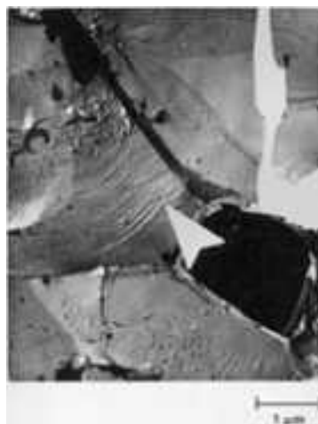
Fig. 15 Wallner lines (arrow) on the surface of a fractured WC-Co specimen. TEM formvar replica. Etched with 5% HCl. (S.B. Luyckx, University of the Witwatersrand)
