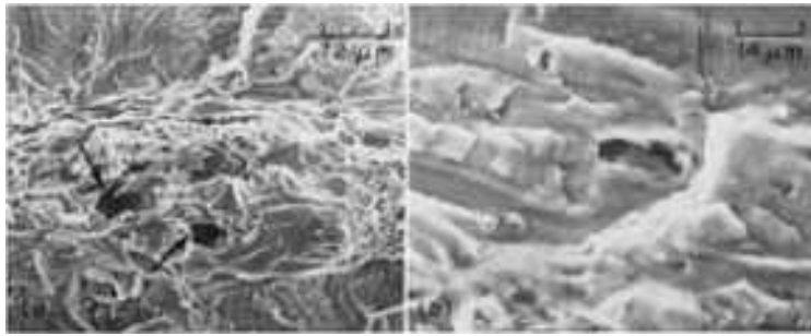
Fig. 111 Fatigue fracture surface of a resistance spot weld that broke during bond testing of an aluminum alloy 7075-T6 specimen. (a) Note voids (arrows) caused by molten-metal shrinkage in the weld nugget. (b) Both fatigue striations and shrinkage voids are evident, which indicates that the fracture path favored the porous areas.
