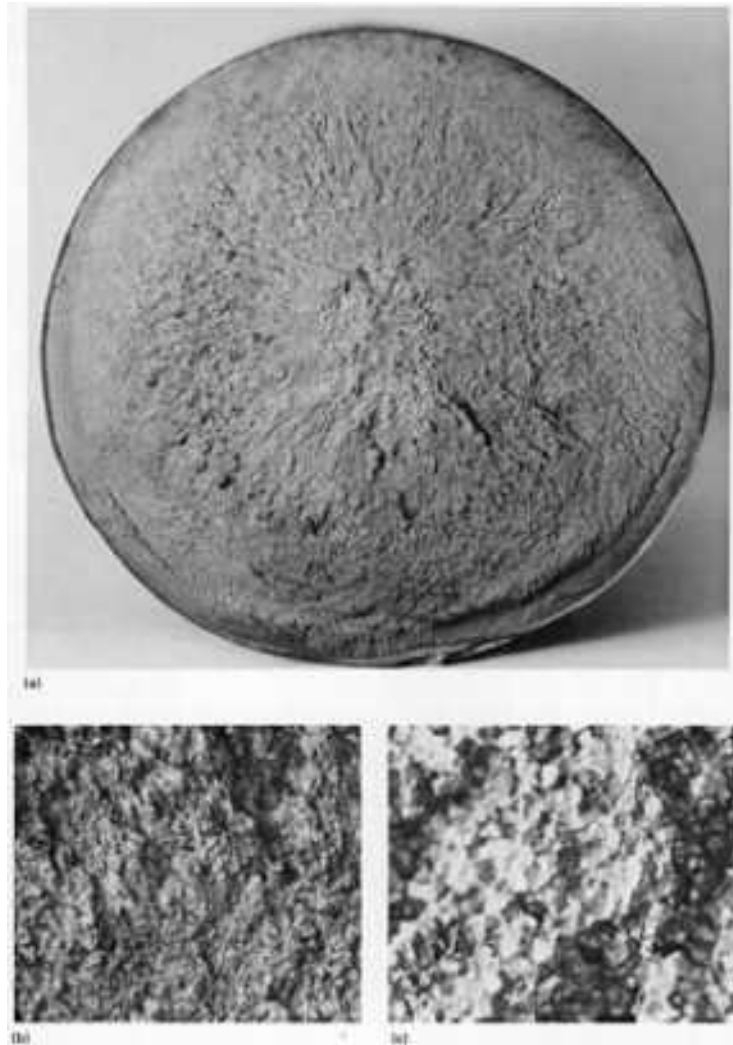
Fig. 115 AISI 1070 steel bar that broke during heat treatment due to gross chemical segregation. (a) Macrograph at actual size. (b) Fracture near the outside surface of the bar. 8 \times . (c) Fracture near the center of the bar. 8 \times . Note the coarse grain structure of the center region.
