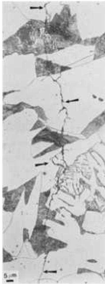
Fig. 72 Fatigue crack (arrows) in a ferrite-pearlite microstructure in a carbon steel. Etched with 2% nital. 800×
