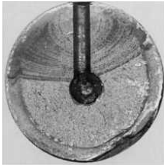
Fig. 219 Fractograph of fatigue failure in SAE 1050 pin, induction hardened to a depth of 5 mm ( \frac{3}{16} in.) and surface hardness of 55 HRC. Core hardness: 21 HRC. Fatigue initiated inside the grease hole at the metallurgical notch created by the very sharp case-core hardness gradient. 1.8× (K. Marden, California Polytechnic State University)
