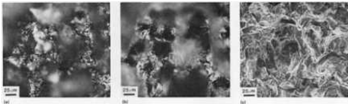
Fig. 11 Comparison of light microscope (a and b) and SEM (c) images of a ductile fracture in an alloy X-750
