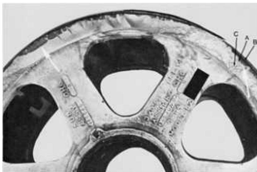
Fig. 1196 Portion of an aircraft landing wheel of sand-cast magnesium alloy AZ81A-T4, showing a corrosion-fatigue fracture that occurred in service at the locking-ring channel. Nominal tensile strength was 276 MPa (40 ksi). The fracture extended halfway around the perimeter of the wheel. Many discolored, crescent-shaped fatigue-crack nuclei were found; two are indicated by white arrows. See Fig. 1197, 1198, 1199, and 1200 for TEM views of areas at A, B, and C. 0.3×
