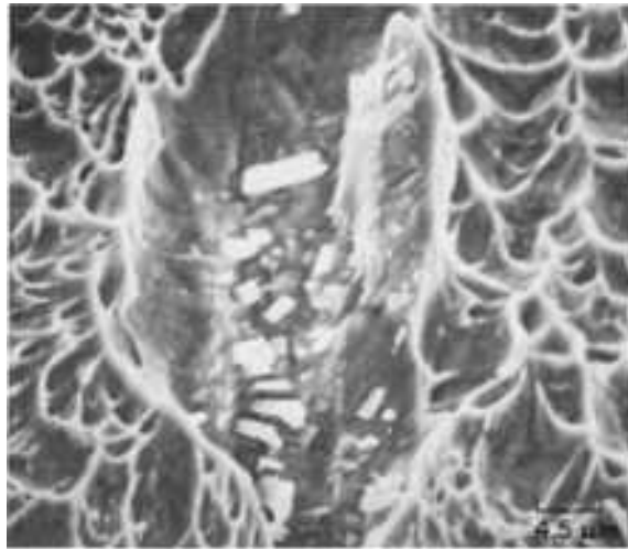
Fig. 801 Higher-magnification view of the area in the rectangle in Fig. 800, showing one of the very large voids. Clearly visible is the array of Ti(C,N) inclusions that triggered the formation of this void. These may have been separate particles originally, or they may be segments of one or more larger particles that broke apart before the void opened. Except for a few tiny dimples visible here (lower right), the region in Fig. 800 was found to lack the dispersion of fine dimples normally present in surfaces of tensile-test fractures. SEM, 2200×
