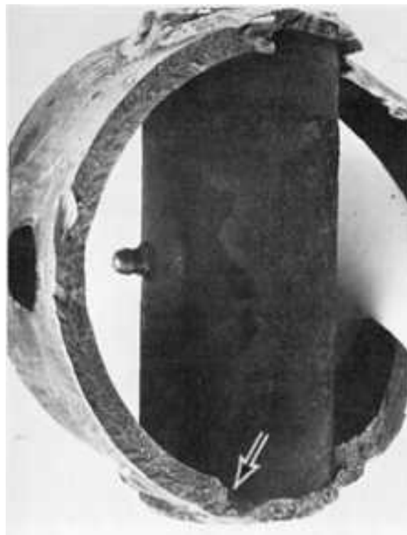
Fig. 186 View of the top segment of the fractured pressure-vessel shell in Fig. 177, showing an area of the fracture surface just to the right of the crack nucleus. Note that here the chevron marks clearly point to the left, toward the fracture origin. The crack ends at far right, where a section was removed for testing. 0.28\times
