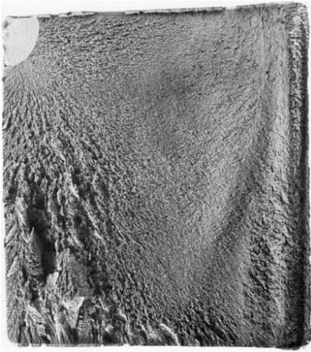
Fig. 571 Surface of a fracture in an equalizer bar, which supports the front end of a tractor, fabricated from D6B steel and heat treated to a hardness of 45 to 47 HRC. The bar was put into service for 200 h and then returned to the laboratory, where it was flexed in fatigue to fracture at 60 \times 10^3 cycles. Note the very fine texture of the fatigue-crack zone at the upper left corner. It is concluded that because there are no beach marks beyond that small corner zone, the remainder of the fracture occurred in a catastrophic manner. Shear lips are evident along the top and right edges, and may also be present around the lower left corner. (D6B steel contains 0.45% C, 0.80% Mn, 1.00% Cr, 0.50% Ni, 1.00% Mo, and 0.10% V.) ~1.13×
