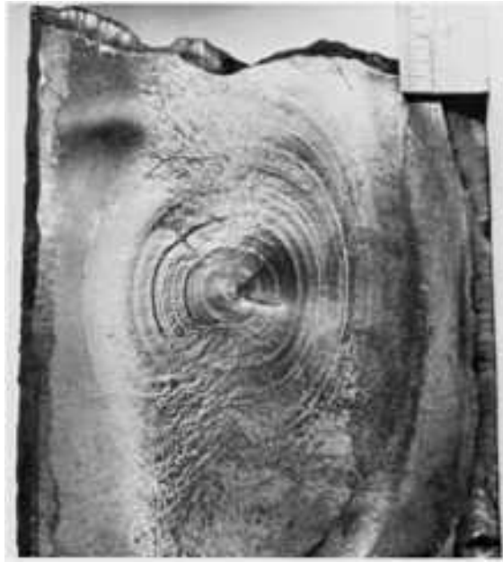
Fig. 258 Surface of a fatigue fracture that developed in the flange of an AISI 1055 steel wheel of an open-hearth crane after nearly 20 years of service. The fracture surface was exposed by arc cutting the adjacent metal. This fatigue fracture, like the one shown in Fig. 257, was initiated by an internal flaw and propagated outward radially; no external defect was found to be involved in either this fracture in Fig. 257. 0.44×
