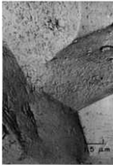
Fig. 398 TEM p-c replica taken from area A (the quench-crack crescent) in the impact fracture surface shown in Fig. 397. Here, the crack is completely intergranular in nature, having faithfully followed the grain interfaces. Traces of oxidation are evident. See also Fig. 399 and 400. 6500×
