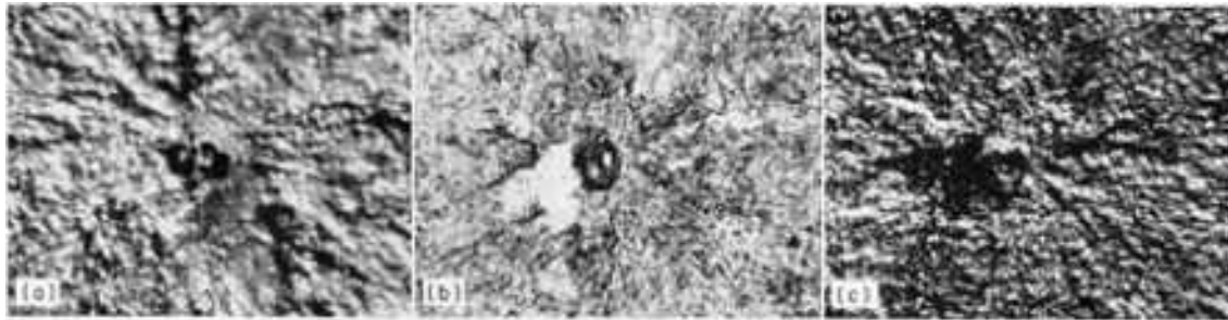
Fig. 14 Comparison of replica fractographs of a fatigue fracture in an induction-hardened 15B28 steel shaft. Fracture was initiated at the large inclusion in the center of the views during rotating bending. (a) Oblique illumination from a point source lamp. (b) Same area as (a), photographed using transmitted light. (c) Replica shadowed with a vapor-deposited coating and photographed using oblique illumination from a point source lamp. All 30×
