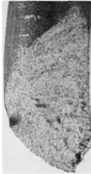
Fig. 268 Fracture surface of the spring in Fig. 267. The fatigue-crack origin is at the seam at left edge. The surface of the wire was gouged after fracture. 3×
