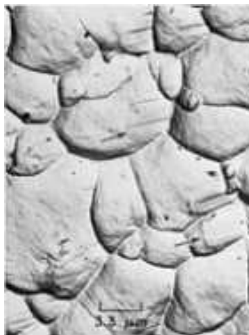
Fig. 7 Scraping artifacts (as at arrows) which resemble linear striations, on the sides of dimples. TEM plastic-carbon replica. 3000×
