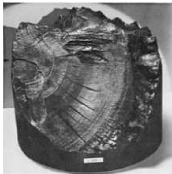
Fig. 152 Fracture surface of a carbon steel drive shaft of a 180-Mg (200-gross-ton) marine tug. The shaft failed by corrosion fatigue after seawater displaced the lubricant between the shaft and the stern tube. Beach marks indicate that the fracture origin was at left (arrow). See also Fig. 153, 154, 155, and 156. 0.8 \times
