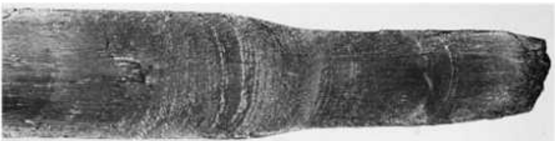
Fig. 206 Mating fracture surface to the one shown in Fig. 205. This piece of the shaft broke away during service. It is believed that the crack propagated a long distance in the longitudinal direction because of weaknesses associated with the presence of longitudinal bands of elongated manganese sulfide inclusions. ~0.5×
