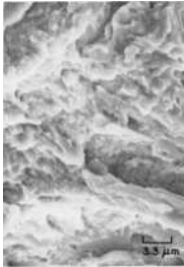
Fig. 566 Higher-magnification view of the area within the rectangle in Fig. 565, which reveals additional small dimples that are not readily apparent at the lower magnification. See Fig. 567, 568, and 569 for the effects of tempering on the fracture surface. SEM, 300×
