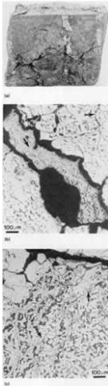
Fig. 85 Hot shortness in a structural steel caused during rolling by internal LME due to copper segregation. (a) Macrograph of section from toe of flange. 0.4 ×. (b) and (c) Micrographs showing grain-boundary copper films that were molten during rolling. (b) and (c) Etched with 2% nital. Both 70×
