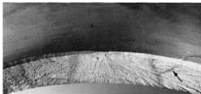
Fig. 413 Surface of a low-cycle fatigue fracture in an aircraft landing-gear cylinder made of AISI 4340 steel that was hardened and tempered to a tensile strength of 1793 to 1931 MPa (260 to 280 ksi). The cylinder was stressed in the laboratory to its tensile strength four times and broke at a stress of 1103 MPa (160 ksi) during the final loading. Note the secondary crack (arrow) to the right of the crack origin (at center), representative of many that extended completely through the wall of the cylinder. See also Fig. 414, 415, 416, and 417. 2×
