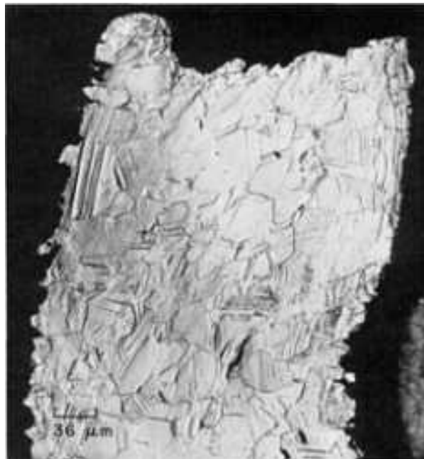
Fig. 920 Longitudinal section through a fatigue fracture in a shute (weft) wire of Fourdrinier wire cloth of 80Cu-20Zn brass with 0.5% Sn added. The profile of the fracture is shown at top. Note corrosion pitting visible on the wire surface at left and at right, \text{FeCl}_3 . 265×
