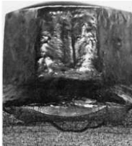
Fig. 209 View of the weld joining the flange and reinforcement plate at top in Fig. 208, showing a crack at the toe of the weld. This crack was present before the fatigue crack, which led to fracture, formed at the toe of the weld in the other flange. See also Fig. 210. 2×
